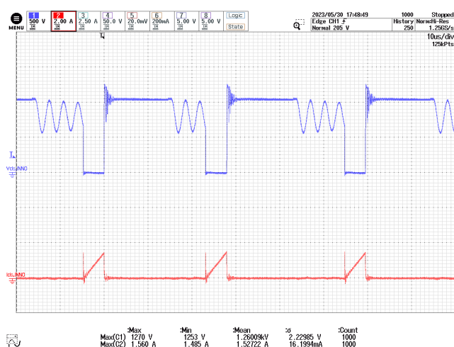
Figure 59 – InnoSwitch3-AQ Drain Voltage and Current. 800 VDC, 6.37 A Load, 25 °C Ambient.
