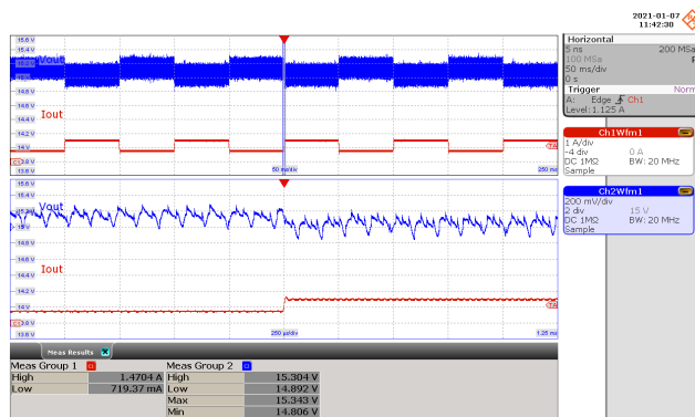
Figure 79 – Transient Response. 132 VAC, 15 V, 0 – 0.75 A Load Step. V_{MIN} : 14.885 V, V_{MAX} : 15.422 V. CH4: V_{OUT} , 0.2 V / div. CH1: I_{LOAD} , 1 A / div. Time: 50 ms / div. (250 \mu s / div. Zoom)
