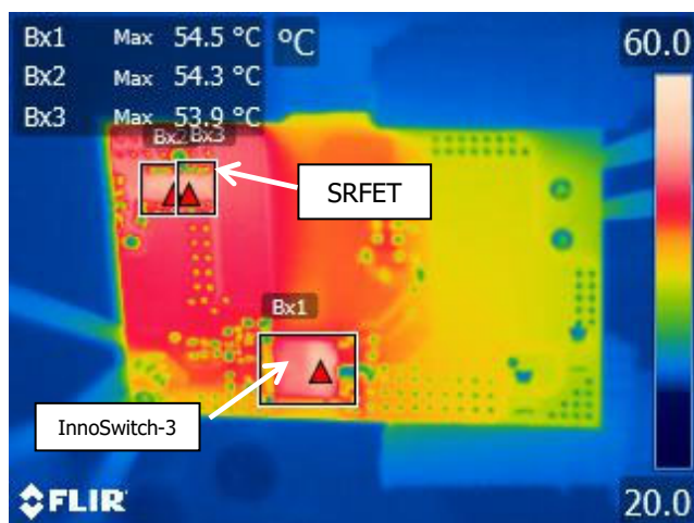
Figure 73 – 400 VDC 1.25 A Full Load. Temperature of INN3996CQ: 54.5 °C. Temperature of SR FET1(Q2): 54.3 °C. Temperature of SR FET2(Q3): 53.9 °C. Ambient Temperature: 28.5 °C.
