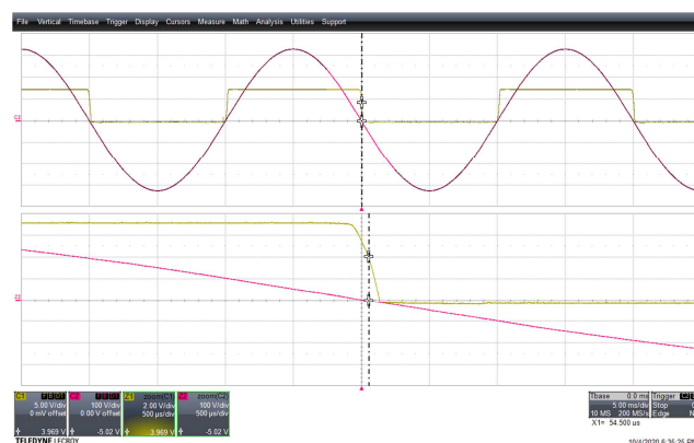
Figure 25 – 230 VAC 50 Hz. CH1: ZCD, 5 V / div., 5 ms / div. CH2: V_{IN} , 100 V / div., 5 ms / div. Rising Edge Delay = 55 μs.
