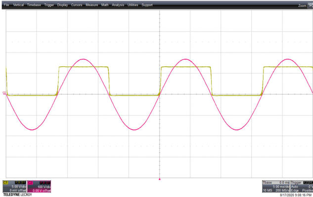
Figure 10 – 120 VAC 60 Hz. CH1: ZCD, 5 V / div., 5 ms / div. CH2: V_{IN} , 100 V / div., 5 ms / div.
