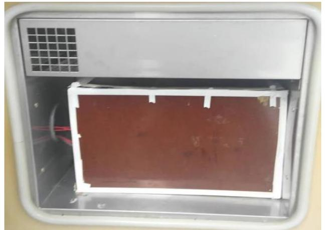
**Figure 105** – Thermal Performance Set-up Using Thermal Chamber.
