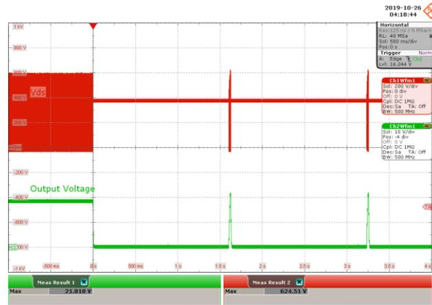
**Figure 75** – 90 VAC 60 Hz, Full load
