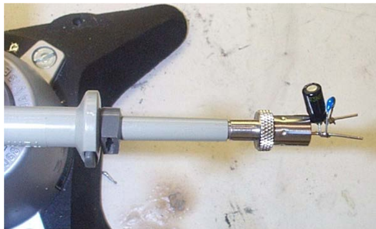
Figure 64 – Oscilloscope Probe with Probe Master ( www.probemaster.com ) 4987A BNC Adapter. (Modified with wires for ripple measurement, and two parallel decoupling capacitors added.)
