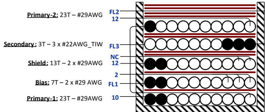
Figure 7 – Transformer Build Diagram.
