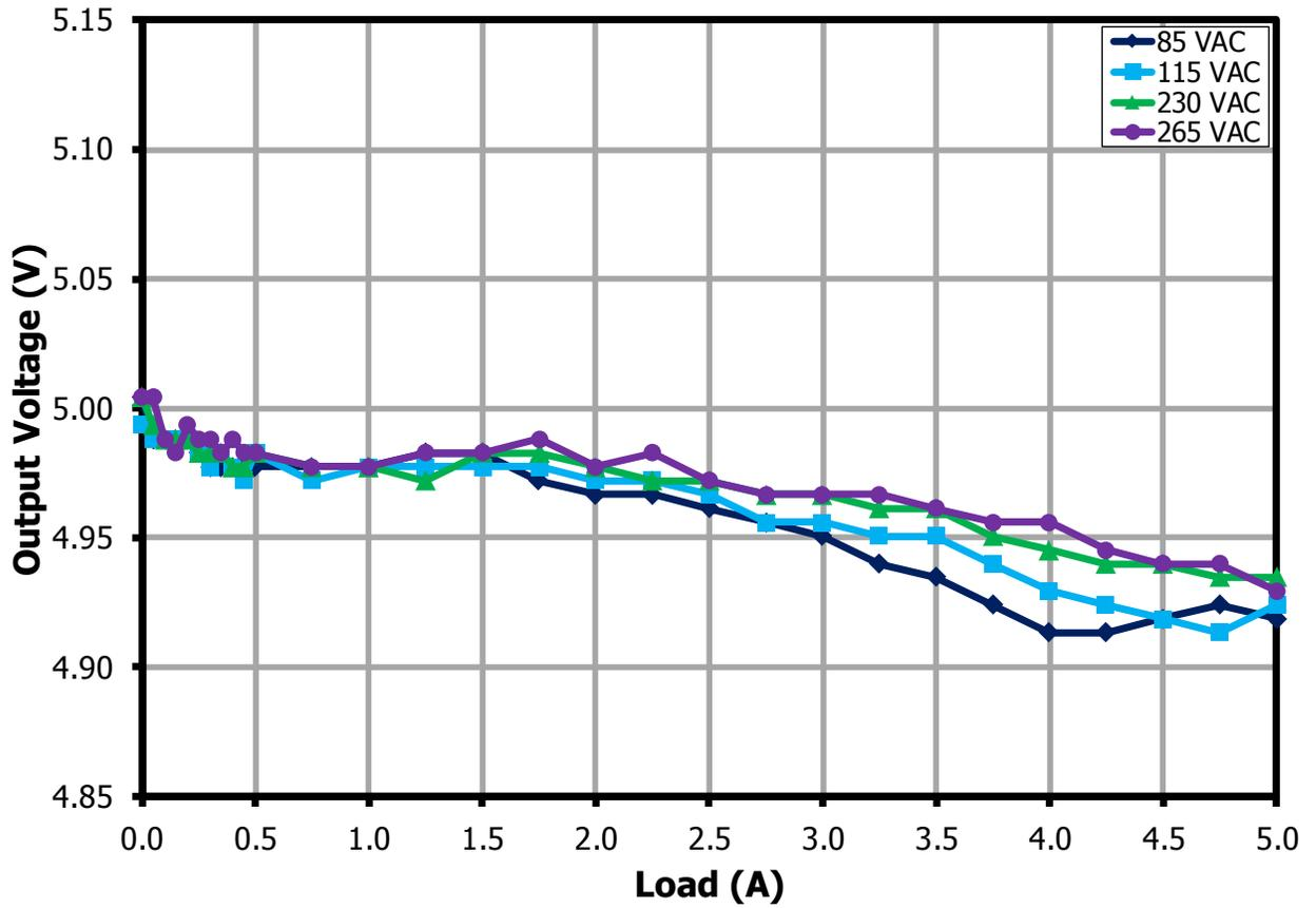
Figure 15 – Load Regulation Measured at the Board Output Terminal.
