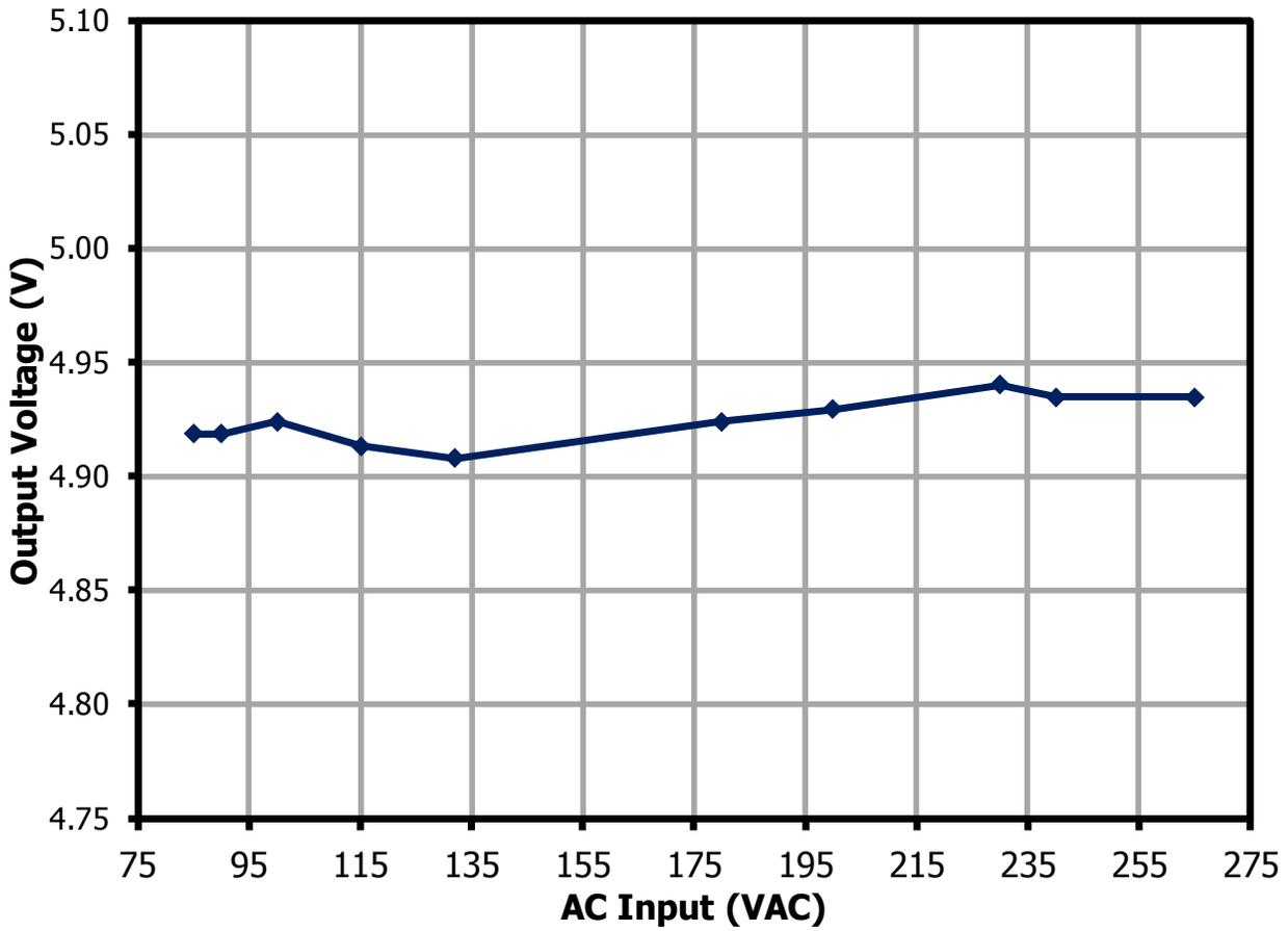
Figure 14 – Line Regulation Measured at the Board Output Terminal.
