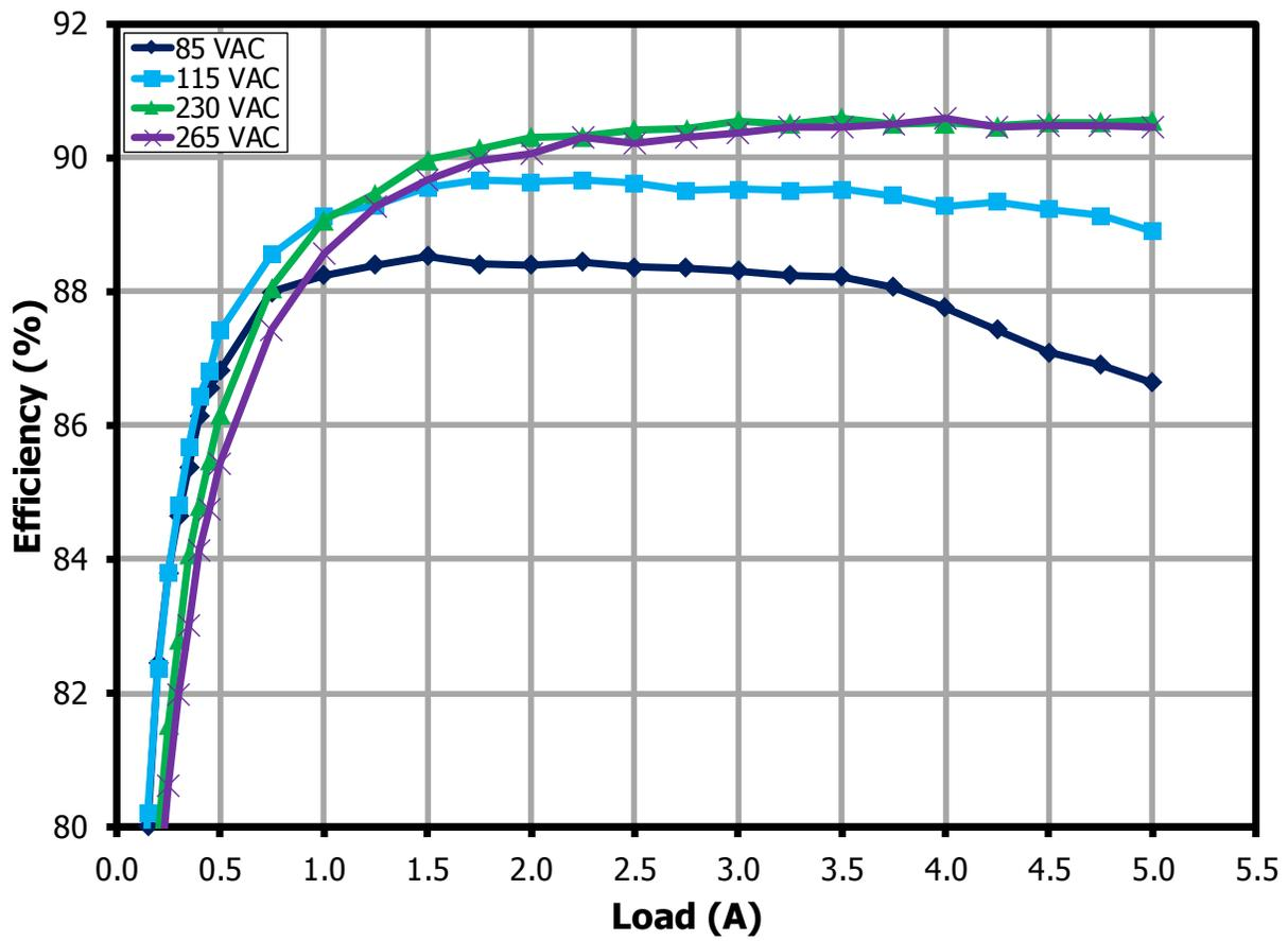
Figure 12 – Efficiency Measured at the Board Output Terminal.
