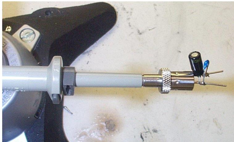
**Figure 17** – Oscilloscope Probe with Probe Master ([www.probemaster.com](http://www.probemaster.com)) 4987A BNC Adapter. (Modified with wires for ripple measurement, and two parallel decoupling capacitors added)
