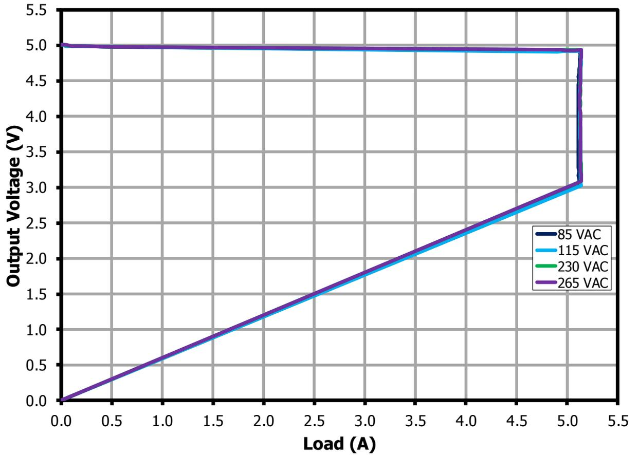
Figure 23 – CV/CC at 25 °C, Measured at the Board Terminal.
