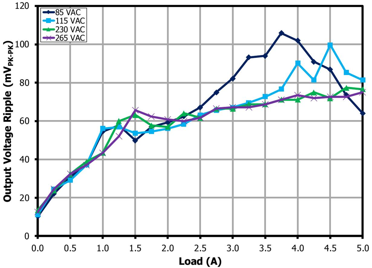
Figure 22 – Output Ripple Measured at the End of a 60 mΩ Cable.
