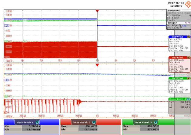
**Figure 50** – Line Undervoltage; DC Input.
