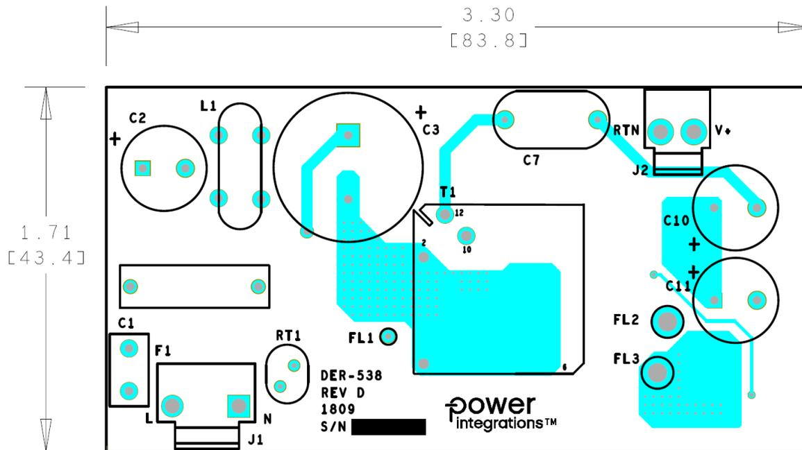
Figure 4 – Printed Circuit Layout, Top.
