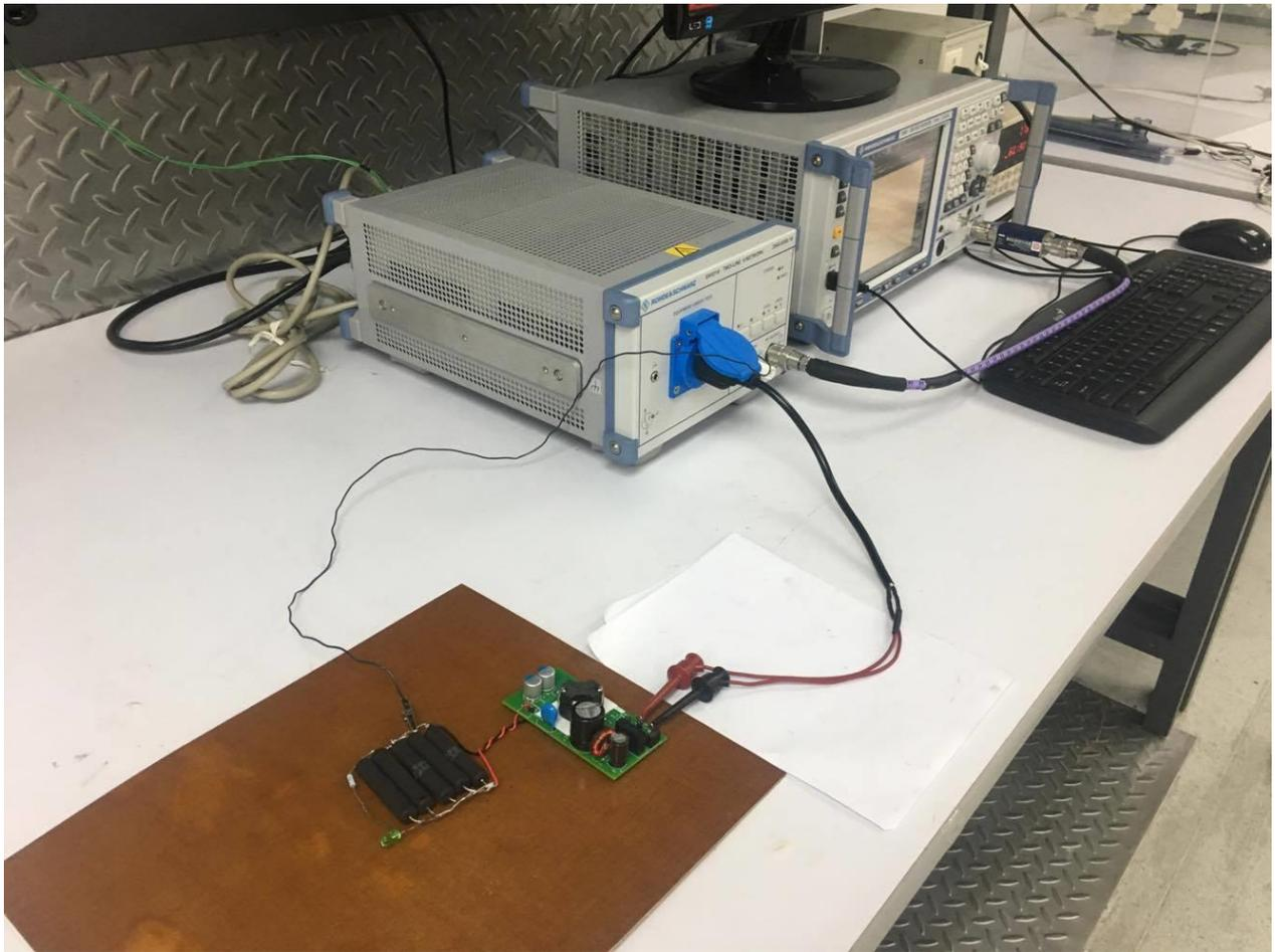
**Figure 54** – Conducted EMI Test Set-up.
