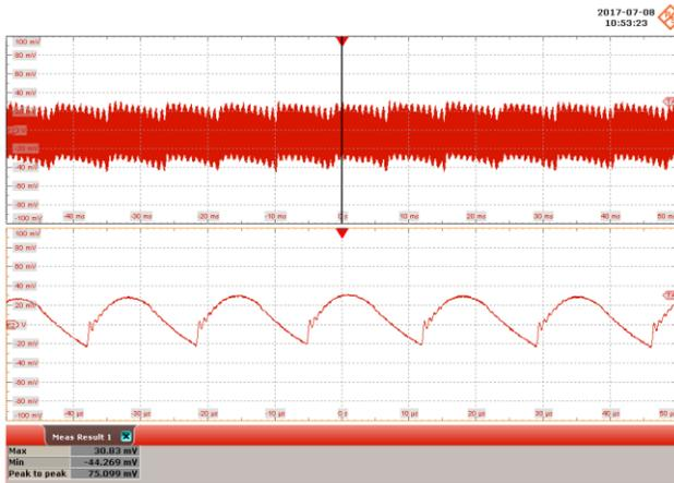
**Figure 18** – 85 VAC, 60 Hz; 100% load.
