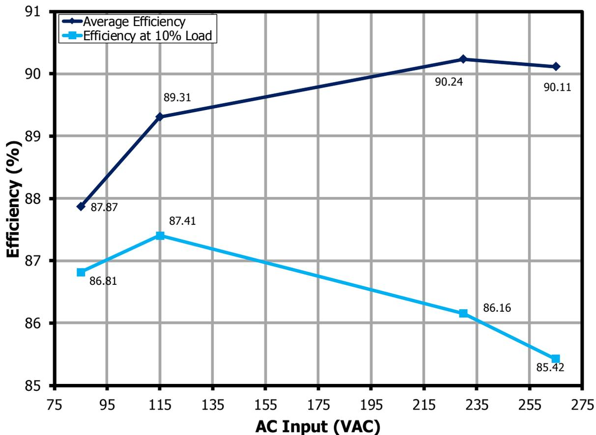
Figure 10 – Efficiency Measured at the Board Output Terminal.
