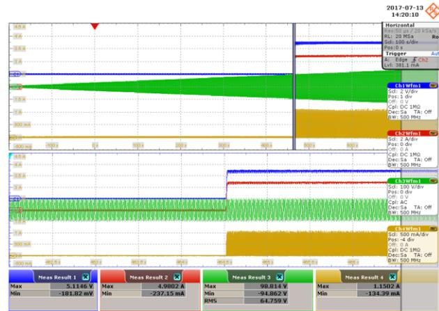
**Figure 52** – Brown-out at No-Load; 90 V to 0 V Input.
