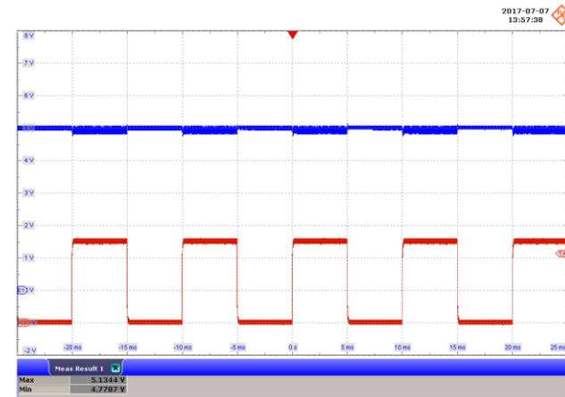
**Figure 43** – 265 VAC, 50 Hz; 0 – 5 A Load Step
