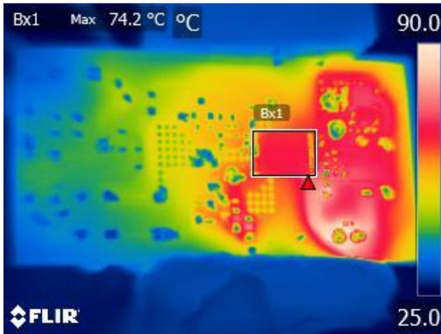
Figure 26 – Bottom Solder Side.
