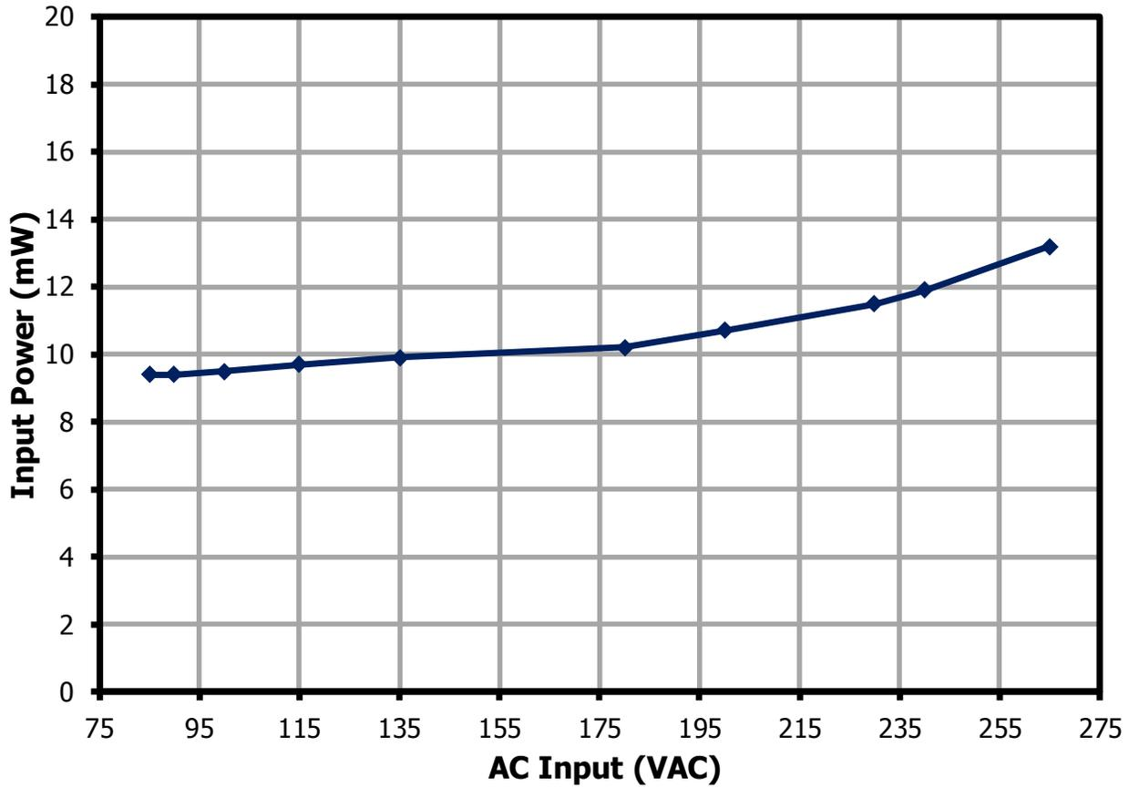
Figure 13 – No-Load Input Power.
