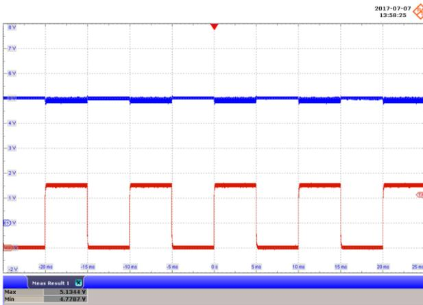
**Figure 42** – 85 VAC, 60 Hz; 0 – 5 A Load Step.
