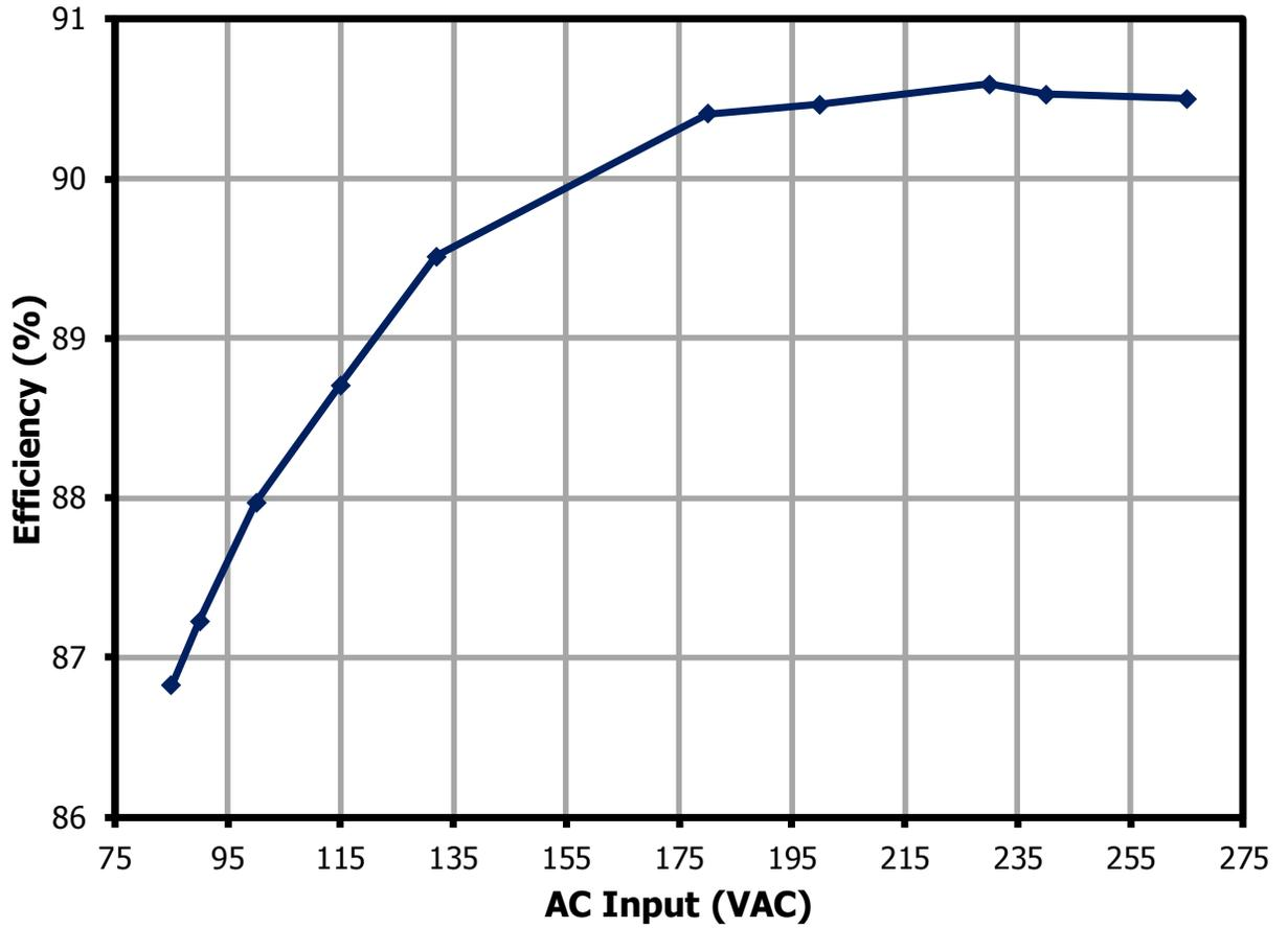
Figure 11 – Efficiency Measured at the Board Output Terminal.
