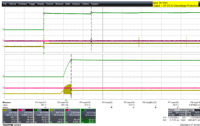
Figure 83 – 85 VAC, No Load – OVP during startup condition.
