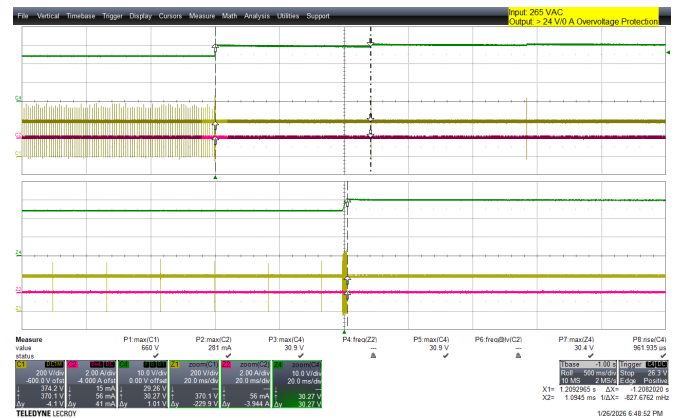
Figure 88 – 265 VAC, No Load – OVP during normal condition.
