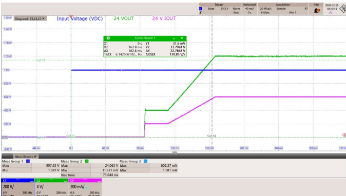
Figure 32 – 24 V Start-up Profile 1000 VDC, Full-Load, Start-up. CH1: V_{IN} , 200 V / div. CH2: V_{OUT\_24V} , 4 V / div. CH3: I_{OUT\_24V} , 200 mA / div. Time Scale: 40 ms / div. t_{ON} Delay: 163 ms
