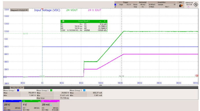
Figure 31 – 24 V Start-up Profile 800 VDC, Full-Load, Start-up. CH1: V_{IN} , 200 V / div. CH2: V_{OUT\_24V} , 4 V / div. CH3: I_{OUT\_24V} , 200 mA / div. Time Scale: 40 ms / div. t_{ON} Delay: 163 ms
