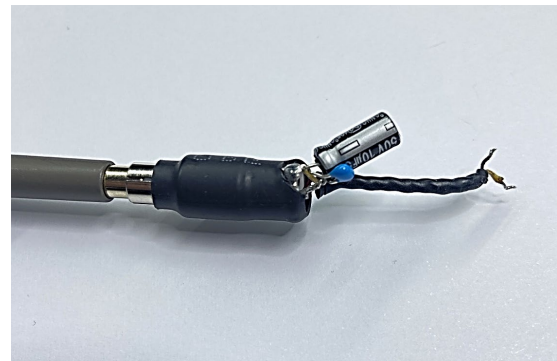
Oscilloscope Probe with Probe Master (www.probemaster.com) 4987A BNC Adapter. (Modified with wires for ripple measurement, and two parallel decoupling capacitors added)
