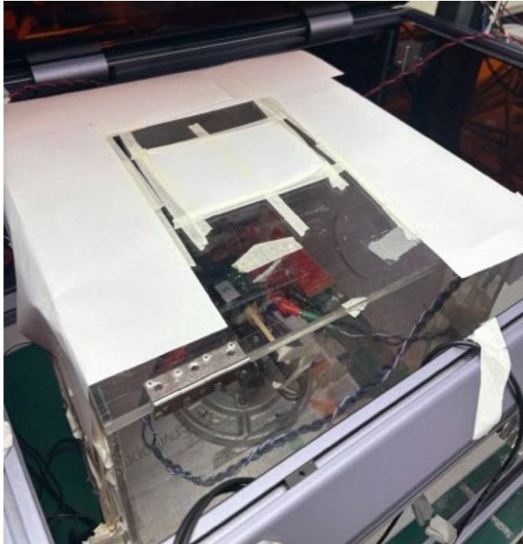
Figure 88 – Thermal Scan Test Set-up.
