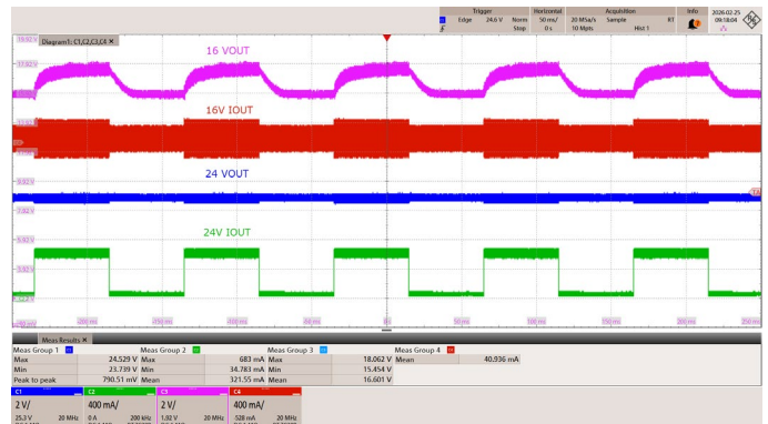
Figure 70 – 800 VDC, Dynamic Load 16 V 35 mA (10%) fixed. 24 V 60 mA (10%) → 600 mA (100%) CH1: V OUT_24V , 2 V / div. CH2: I OUT_24V , 400 mA/div. CH3: V OUT_16V , 2 V / div. CH4: I OUT_16V , 400 mA / div. V OUT(24V)_MAX : 24.5 V V OUT(24V)_MIN : 23.7 V V OUT(16V)_MAX : 18.1 V V OUT(16V)_MIN : 15.5 V
