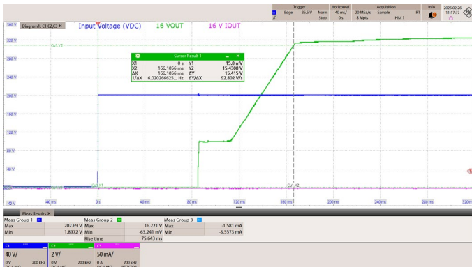
Figure 33 – 16 V Start-up Profile 200 VDC, No-Load, Start-up. CH1: V_{IN} , 40 V / div. CH2: V_{OUT\_16V} , 2 V / div. CH3: I_{OUT\_16V} , 50 mA / div. Time Scale: 40 ms / div. t_{ON} Delay: 166 ms
