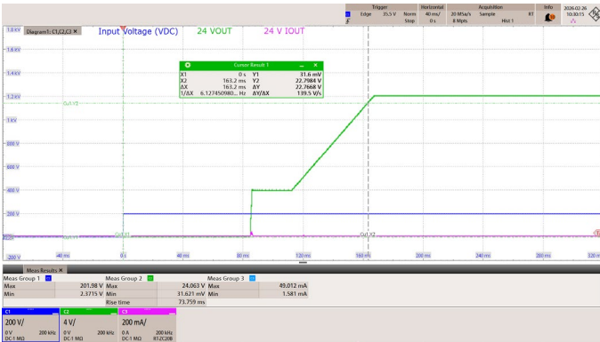
Figure 36 – 24 V Start-up Profile 200 VDC, No-Load, Start-up. CH1: V_{IN} , 200 V / div. CH2: V_{OUT\_24V} , 4 V / div. CH3: I_{OUT\_24V} , 200 mA / div. Time Scale: 40 ms / div. t_{ON} Delay: 163 ms
