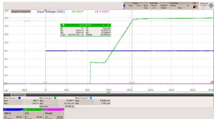
Figure 34 – 16 V Start-up Profile 800 VDC, No-Load, Start-up. CH1: V_{IN} , 200 V / div. CH2: V_{OUT\_16V} , 2 V / div. CH3: I_{OUT\_16V} , 50 mA / div. Time Scale: 40 ms / div. t_{ON} Delay: 165 ms
