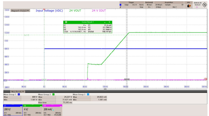
Figure 37 – 24 V Start-up Profile 800 VDC, No-Load, Start-up. CH1: V_{IN} , 200 V / div. CH2: V_{OUT\_24V} , 4 V / div. CH3: I_{OUT\_24V} , 200 mA / div. Time Scale: 40 ms / div. t_{ON} Delay: 162 ms
