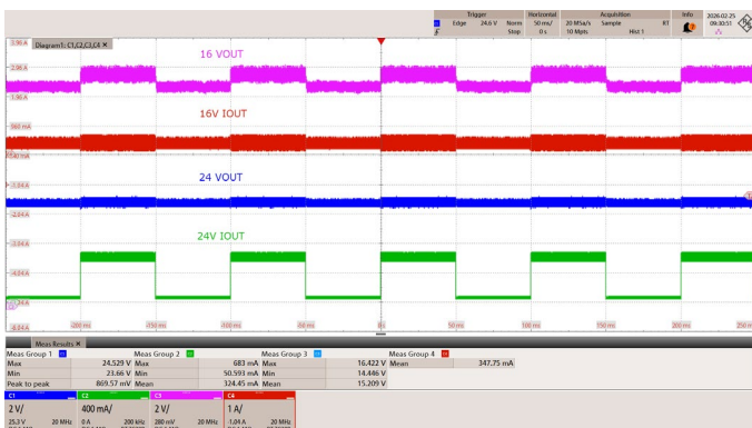
Figure 74 – 1000 VDC, Dynamic Load 16 V 350 mA (100%) fixed. 24 V 60 mA (10%) → 600 mA (100%) CH1: V OUT (24V), 2 V / div. CH2: I OUT (24V), 400 mA/div. CH3: V OUT (16V), 2 V / div. CH4: I OUT (16V), 1 A / div. V OUT (24V)_MAX: 24.5 V V OUT (24V)_MIN: 23.7 V V OUT (16V)_MAX: 16.4 V V OUT (16V)_MIN: 14.5 V
