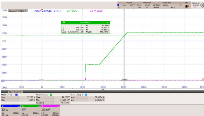
Figure 38 – 24 V Start-up Profile 1000 VDC, No-Load, Start-up. CH1: V_{IN} , 200 V / div. CH2: V_{OUT\_24V} , 4 V / div. CH3: I_{OUT\_24V} , 200 mA / div. Time Scale: 40 ms / div. t_{ON} Delay: 162 ms
