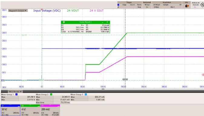
Figure 30 – 24 V Start-up Profile 200 VDC, Full-Load, Start-up. CH1: V_{IN} , 50 V / div. CH2: V_{OUT\_24V} , 4 V / div. CH3: I_{OUT\_24V} , 200 mA / div. Time Scale: 40 ms / div. t_{ON} Delay: 163 ms
