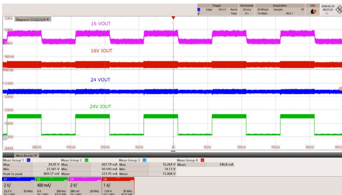
Figure 72 – 200 VDC, Dynamic Load 16 V 350 mA (100%) fixed. 24 V 60 mA (10%) → 600 mA (100%) CH1: V OUT (24V), 2 V / div. CH2: I OUT (24V), 400 mA/div. CH3: V OUT (16V), 2 V / div. CH4: I OUT (16V), 1 A / div. V OUT (24V)_MAX: 24.5 V V OUT (24V)_MIN: 23.6 V V OUT (16V)_MAX: 16.3 V V OUT (16V)_MIN: 14.1 V
