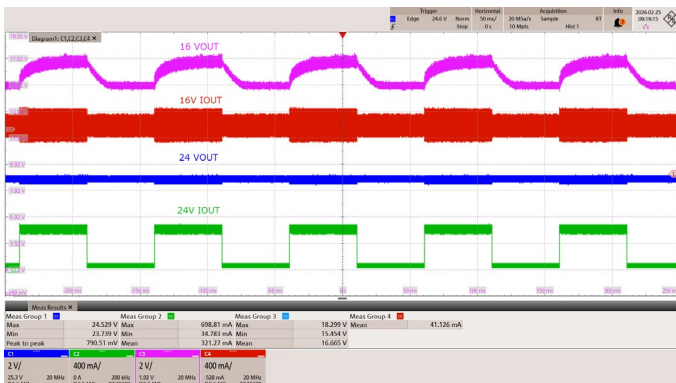
Figure 71 – 1000 VDC, Dynamic Load 16 V 35 mA (10%) fixed. 24 V 60 mA (10%) → 600 mA (100%) CH1: V OUT_24V , 2 V / div. CH2: I OUT_24V , 400 mA/div. CH3: V OUT_16V , 2 V / div. CH4: I OUT_16V , 400 mA / div. V OUT(24V)_MAX : 24.5 V V OUT(24V)_MIN : 23.7 V V OUT(16V)_MAX : 18.3 V V OUT(16V)_MIN : 15.5 V
