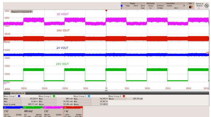
Figure 73 – 800 VDC, Dynamic Load 16 V 350 mA (100%) fixed. 24 V 60 mA (10%) → 600 mA (100%) CH1: V OUT (24V), 2 V / div. CH2: I OUT (24V), 400 mA/div. CH3: V OUT (16V), 2 V / div. CH4: I OUT (16V), 1 A / div. V OUT (24V)_MAX: 24.5 V V OUT (24V)_MIN: 23.7 V V OUT (16V)_MAX: 16.3 V V OUT (16V)_MIN: 14.4 V
