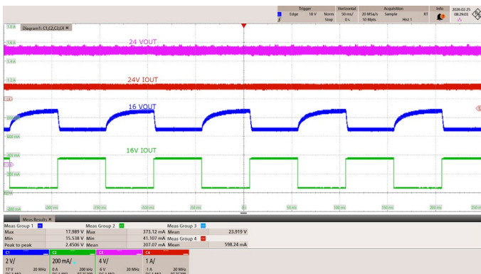
Figure 68 – 1000 VDC, Dynamic Load 16 V 35 mA (10%) → 350 mA (100%) 24 V 600 mA (100%) fixed. CH1: V OUT (16V), 2 V / div. CH2: I OUT (16V), 200 mA/div. CH3: V OUT (24V), 4 V / div. CH4: I OUT (24V), 1 A / div. V OUT (16V) MAX : 18 V V OUT (16V) MIN : 15.5 V
