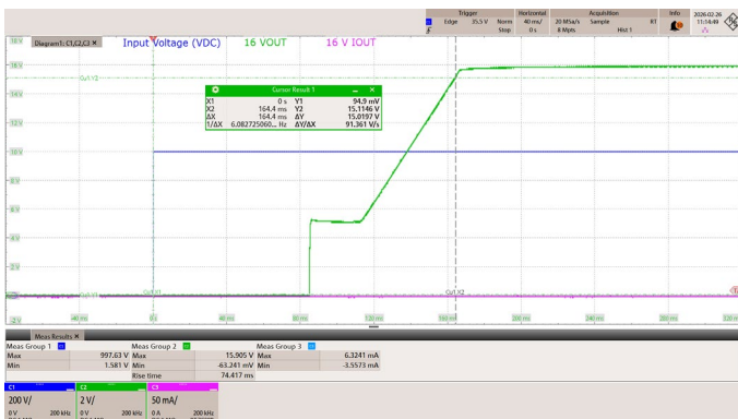
Figure 35 – 16 V Start-up Profile 1000 VDC, No-Load, Start-up. CH1: V_{IN} , 200 V / div. CH2: V_{OUT\_16V} , 2 V / div. CH3: I_{OUT\_16V} , 50 mA / div. Time Scale: 40 ms / div. t_{ON} Delay: 165 ms
