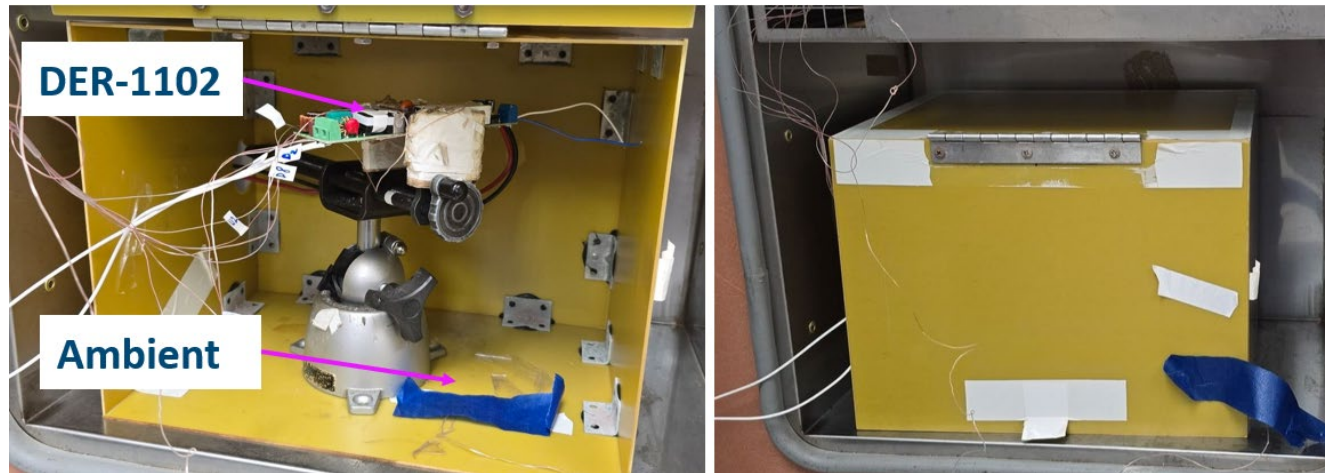
Figure 49 – Thermal Scan Test Set-up at 55 °C Ambient.
