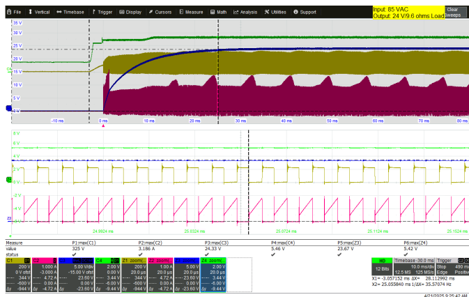
Figure 26 – 85 VAC, 60 Hz, 24 V / 2.5 A. CH1: TOP7074K_V DS , 200 V / div., 10 ms / div. CH2: TOP7074K_I DS , 1 A / div., 10 ms / div. CH3: V OUT , 5 V / div., 10 ms / div. CH4: V BP , 2 V / div., 10 ms / div. Zoom: 20 μs / div. Output Voltage, max = 24.3 V Start-up time = 25 ms
