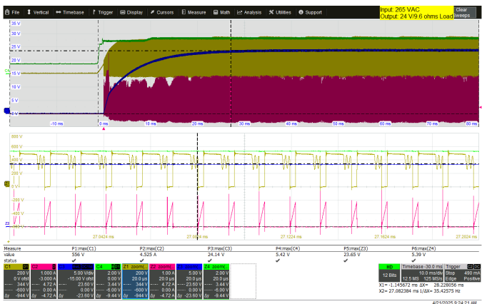
Figure 27 – 265 VAC, 50 Hz, 24 V / 2.5 A. CH1: TOP7074K_V DS , 200 V / div., 10 ms / div. CH2: TOP7074K_I DS , 1 A / div., 10 ms / div. CH3: V OUT , 5 V / div., 10 ms / div. CH4: V BP , 2 V / div., 10 ms / div. Zoom: 20 μs / div. Output Voltage, max = 24.1 V Start-up time = 27 ms
