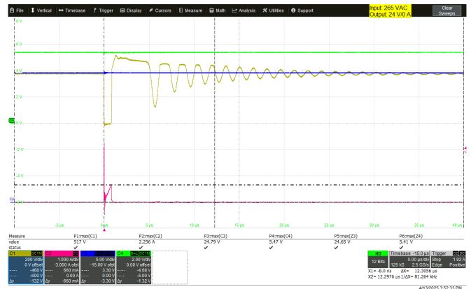
Figure 33 – 265 VAC, Io = 0 A (No-Load).
