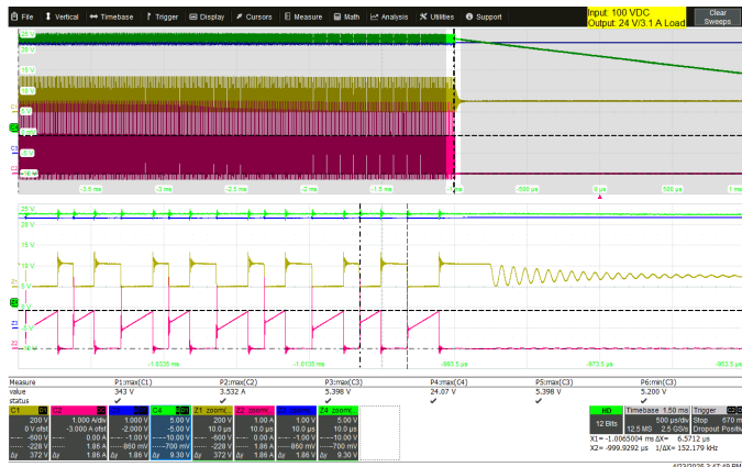
Figure 77 – 100 VDC, I o = 3.1 A (74.4 W). CH1: TOP7074K_V DS , 200 V / div., 500 μs / div. CH2: TOP7074K_I DS , 1 A / div., 500 μs / div. CH3: V BP , 1 V / div., 500 μs / div. CH4: V OUT , 5 V / div., 500 μs / div. Zoom: 10 μs/div. F S = 152 kHz I LIM = 1.86 A
