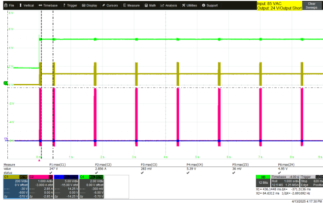
Figure 75 – 85 VAC, Startup Output Short. CH1: TOP7074K_V DS , 200 V / div., 500 ms / div. CH2: TOP7074K_I DS , 1 A / div., 500 ms / div. CH3: V OUT , 5 V / div., 500 ms / div. CH4: V BP , 2 V / div., 500 ms / div Zoom: 20 ms/div. V DS max = 247 V, 34% derating I DS max = 2.86 A t AR(ON) = 74 ms t AR(OFF) = 1.22 s t AR(OFF)H = 371 ms
