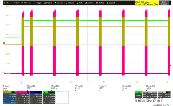
Figure 76 – 265 VAC, Startup Output Short. CH1: TOP7074K_V DS , 200 V / div., 500 ms / div. CH2: TOP7074K_I DS , 1 A / div., 500 ms / div. CH3: V OUT , 5 V / div., 500 ms / div. CH4: V BP , 2 V / div., 500 ms / div Zoom: 20 ms/div. V DS max = 572 V, 78.9% derating I DS max = 6.66 A t AR(ON) = 368 ms t AR(OFF) = 1.25 s t AR(OFF)H = 371 ms
