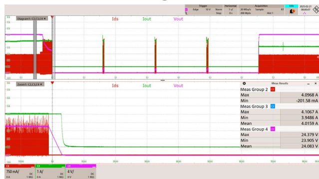
Figure 155 – 198 VAC, 50 Hz. 24 V / 4 A Over-current
