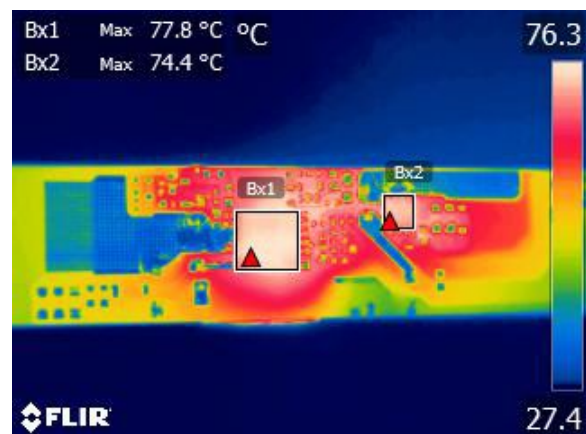
Figure 50 – Thermal Scan 305 V 24 V / 3.13 A Bx1: U3-Pri (INN4274C): 77.8 °C Bx2: Q3-Sec (SR FET): 74.4 °C Ambient: 27.4 °C
