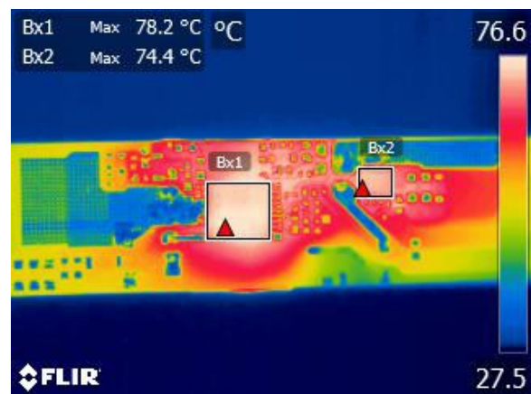
Figure 46 – Thermal Scan 277 V 24 V / 3.13 A Bx1: U3-Pri (INN4274C): 78.2 °C Bx2: Q3-Sec (SR FET): 74.4 °C Ambient: 27.5 °C
