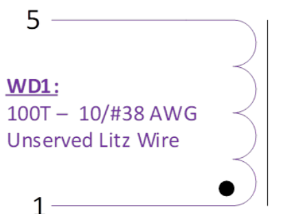
Figure 10 – Boost Inductor Electrical Diagram.
