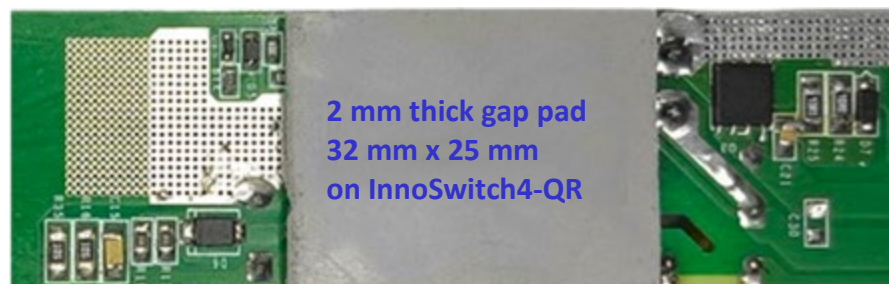
Figure 20 – INS1: InnoSwitch4-QR IC Gap Pad Setup on DER-1061 (Bottom View).
