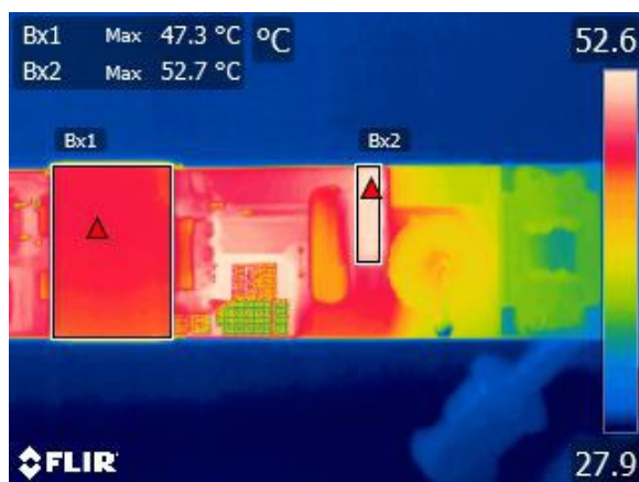
Figure 47 – Thermal Scan 277 V 24 V / 3.13 A Bx1: T3-(PFC Inductor): 47.3 °C Bx2: BR1-(Rectifier): 52.7 °C Ambient: 27.9 °C
