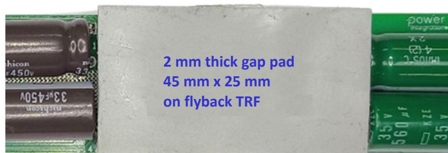
Figure 21 – INS2: Flyback TRF Gap Pad Setup on DER-1061 (Top View).
