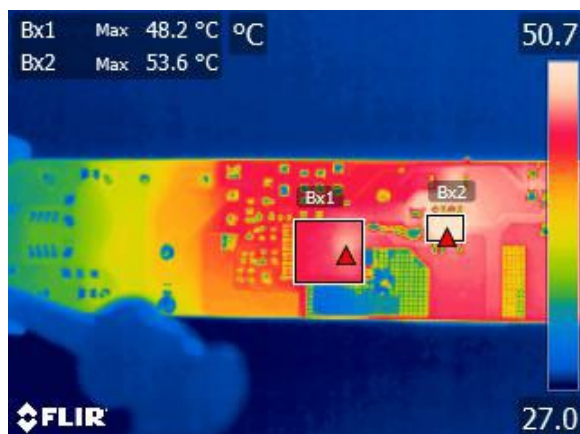
Figure 49 – Thermal Scan 305 V 24 V / 3.13 A Bx1: U2-(PFS7623C): 48.2 °C Bx2: D1-(Boost Diode): 53.6 °C Ambient: 27.0 °C
