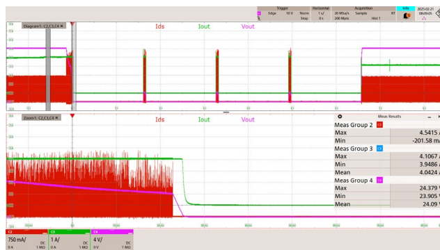
Figure 156 – 305 VAC, 50 Hz. 24 V / 4 A Over-current
