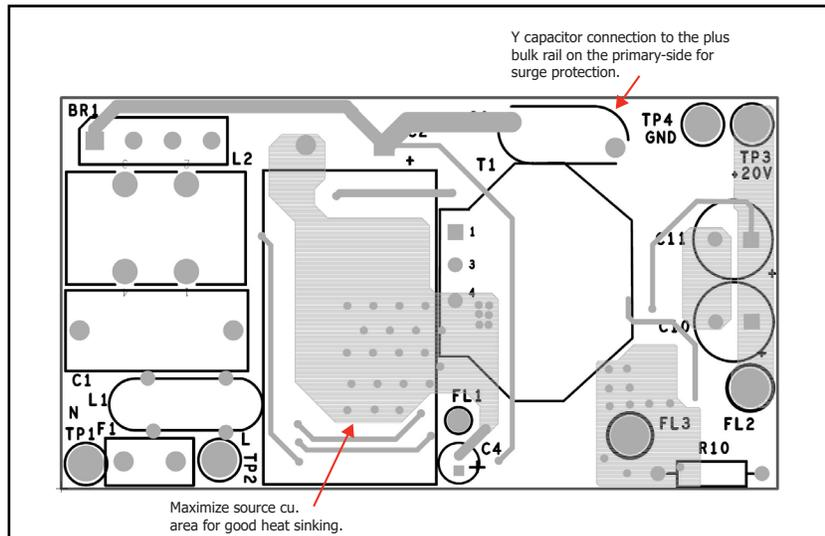
Figure 6. PCB Layout Top Side.
