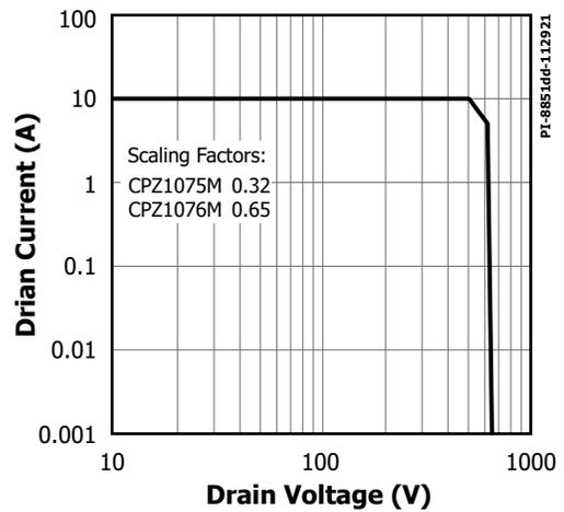
Figure 17. Maximum Allowable Drain Current vs. Drain Voltage.
