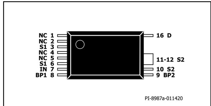
Figure 4. Pin Configuration.
