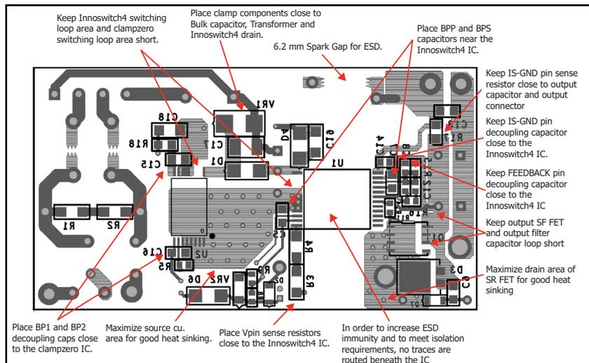
Figure 7. PCB Layout Bottom Side.
