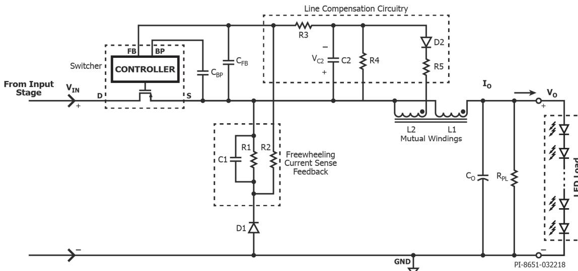
Figure 2. The Input Line Regulation Circuitry Implemented Through a Winding on the Inductor.
