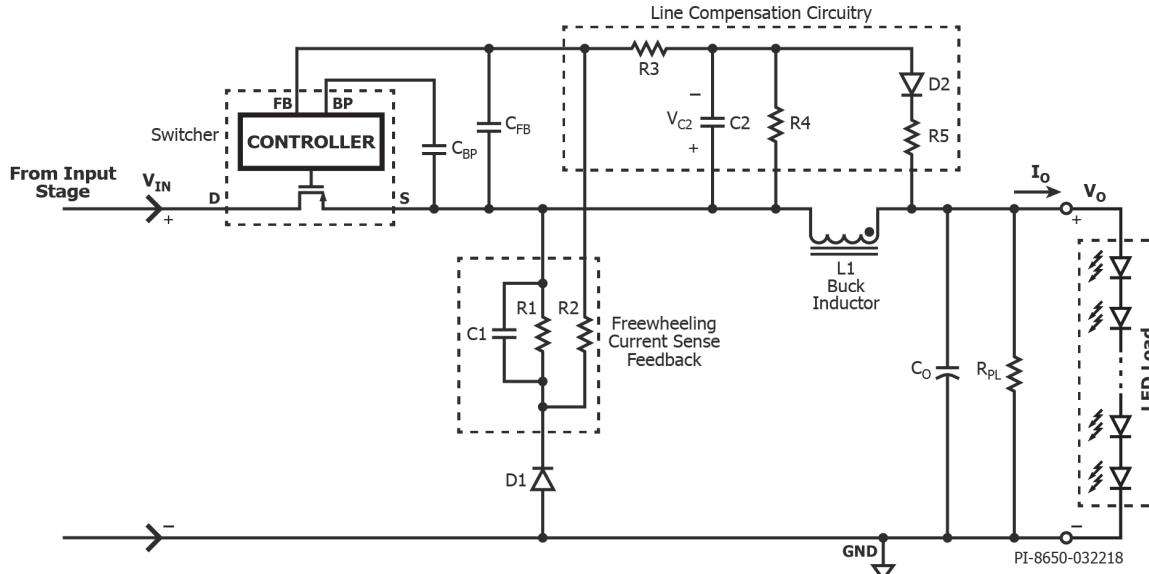
Figure 1. Example of the Input Line Regulation Circuitry Implemented in a Buck Converter with High-Side Switching.
