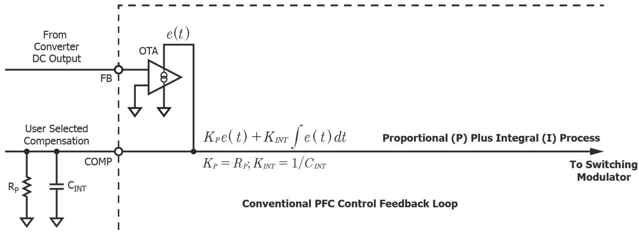
Figure 1. The Conventional PFC Control Feedback Loop with a Simple Proportional (P) Plus Integral (I) Process.
