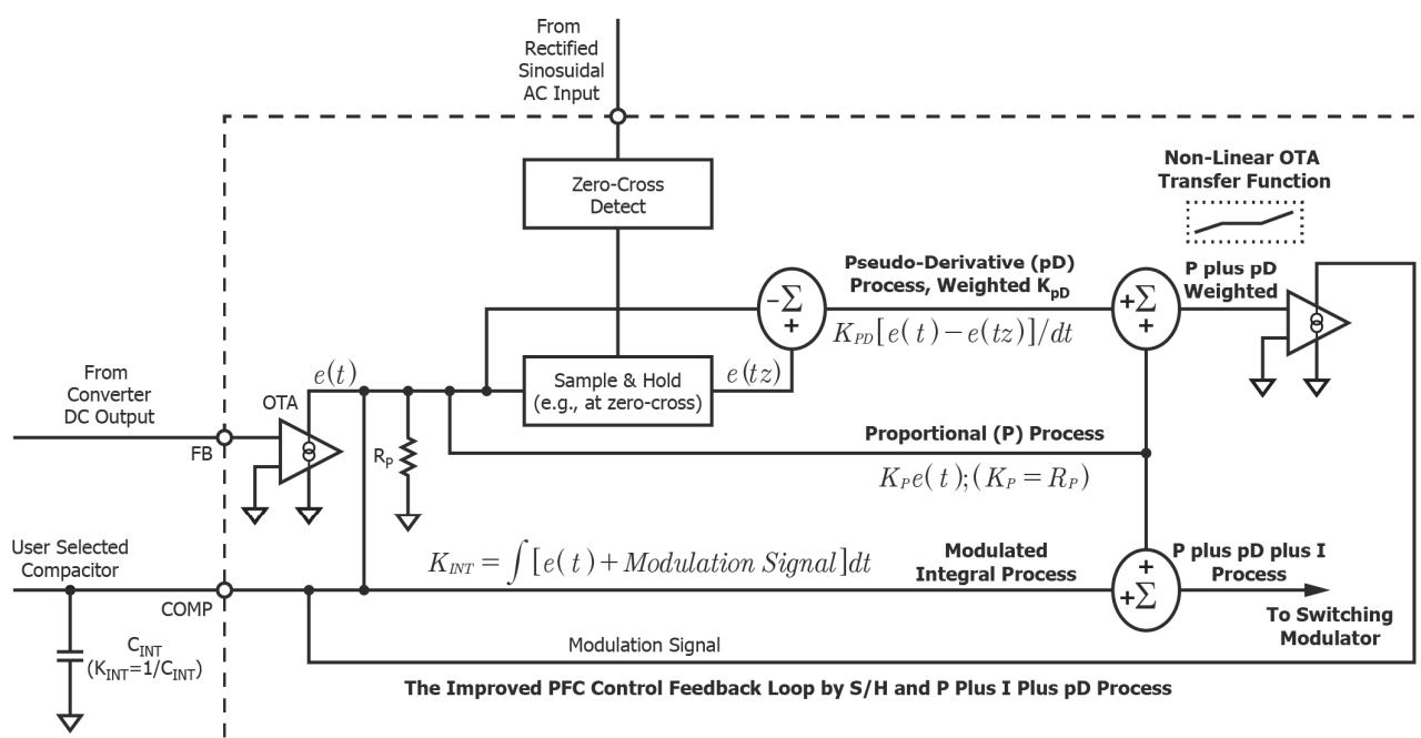
Figure 2: Improved PFC Control Feedback Loop by Using Sample-hold (S/H) and Control Processes Including Proportional (P) plus Integral (I) plus Pseudo-Derivative (pD).
