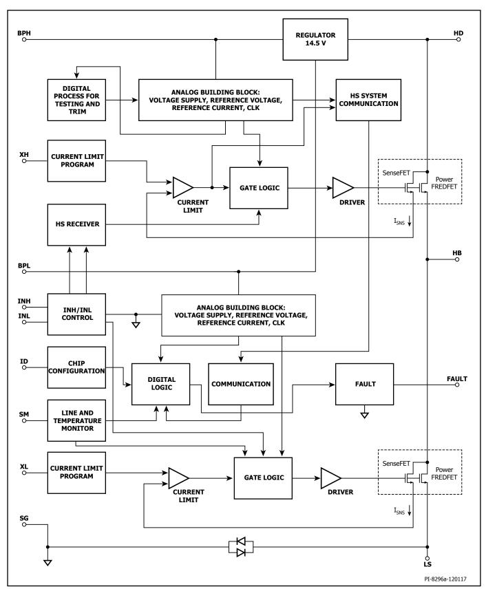
Figure 3. Functional Block Diagram BRD116X.
