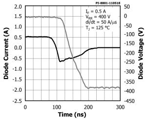
Figure 27. Typical Diode Reverse Recovery (BRD1X60).
