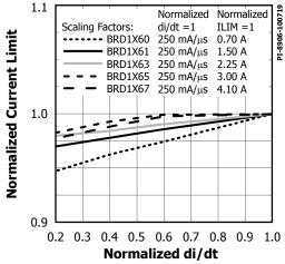
Figure 34. Default Current Limit vs. di/dt.
