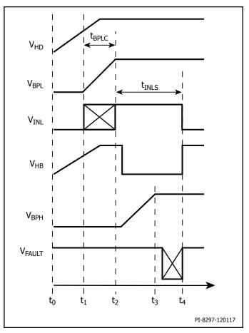
Figure 9. Recommended Power-Up Sequence with Self-supplied Operation.
