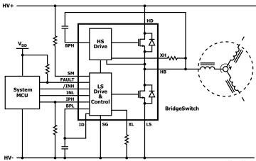
Figure 1. Typical 3-Phase Inverter Schematic (BRD126X).
