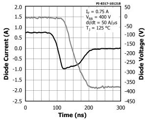
Figure 28. Typical Diode Reverse Recovery (BRD1X61).
