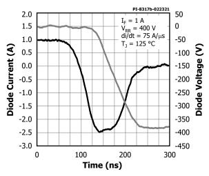
Figure 31. Typical Diode Reverse Recovery (BRD1X67).
