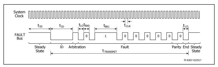
Figure 21. Status Communication Bit Stream.
