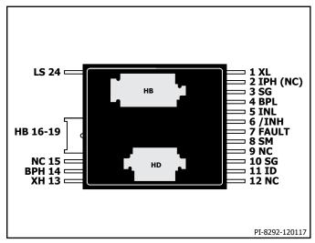
Figure 5. Pin Configuration (Bottom View).
