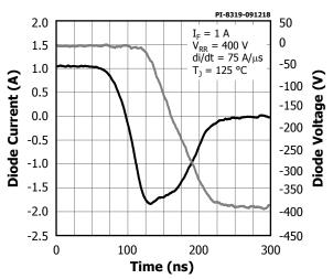
Figure 30. Typical Diode Reverse Recovery (BRD1X65).
