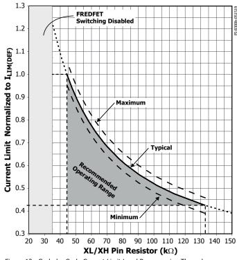
Figure 12. Cycle-by-Cycle Current Limit Level Programming Through EXTERNAL CURRENT LIMIT Pin.
