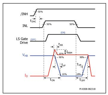
Figure 23. Low-Side FREDFET Switching Timing.
