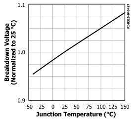
Figure 25. Power FREDFET Breakdown vs. Temperature.
