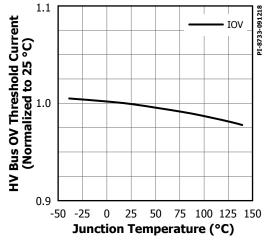
Figure 38. HV Bus OV Threshold Current vs. Temperature.
