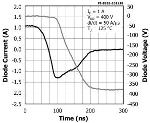
Figure 29. Typical Diode Reverse Recovery (BRD1X63).
