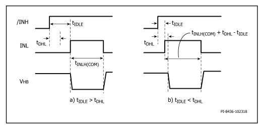
Figure 24. Minimum INL High Time Required for Device Internal High-Side Status Update a)  $t_{\text{IDLE}} > t_{\text{DHL}}$  b)  $t_{\text{IDLE}} < t_{\text{DHL}}$ .
