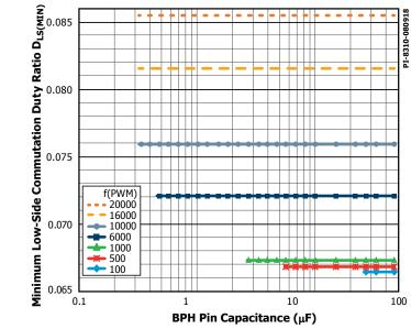
Figure 8. Minimum Low-Side Commutation Duty Ratio vs. BYPASS HIGH-SIDE Pin Capacitance and Low-Side PWM Frequency to Ensure Sufficient High-Side Self-Supply Current (High-Side Commutation Duty Ratio  $\leq$  0.95).
