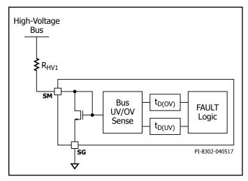
Figure 15. High-Voltage Bus Monitoring with SYSTEM MONITOR Pin.
