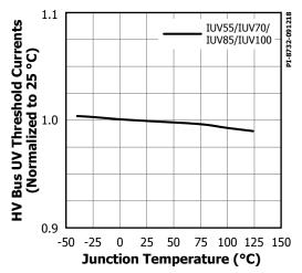
Figure 37. HV Bus UV Threshold Current vs. Temperature.
