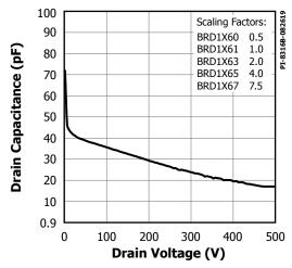
Figure 26. Power FREDFET C<sub>oss</sub> vs. Voltage.
