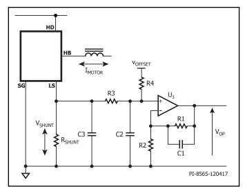
Figure 14. External Current Sense Example Circuit (BRD116X).
