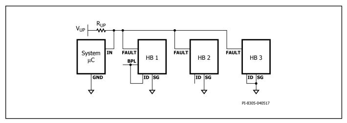
Figure 19. Single Wire Status Communication Bus with Device ID Programming.
