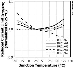
Figure 33. Reducted Current Limit vs. Temperature.
