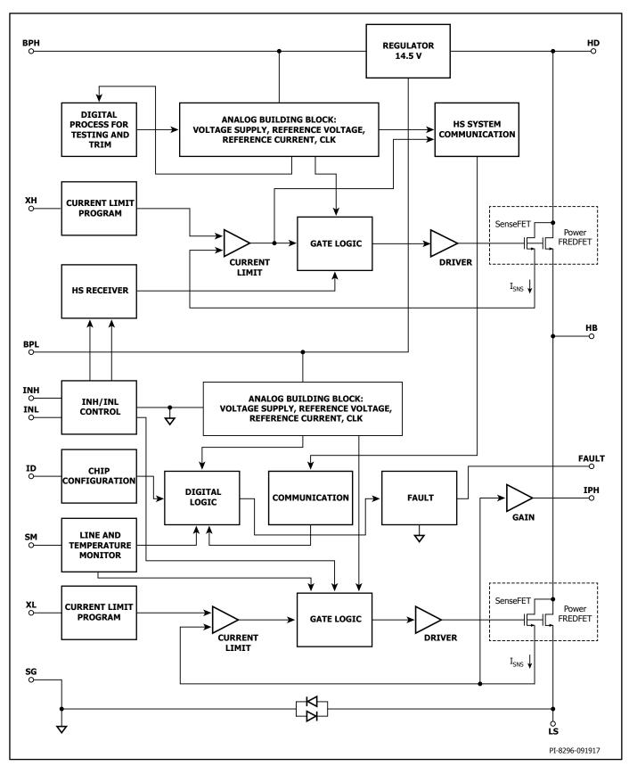
Figure 4. Functional Block Diagram BRD126X.
