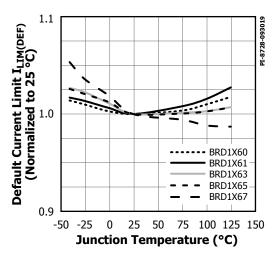
Figure 32. Default Current Limit vs. Temperature.
