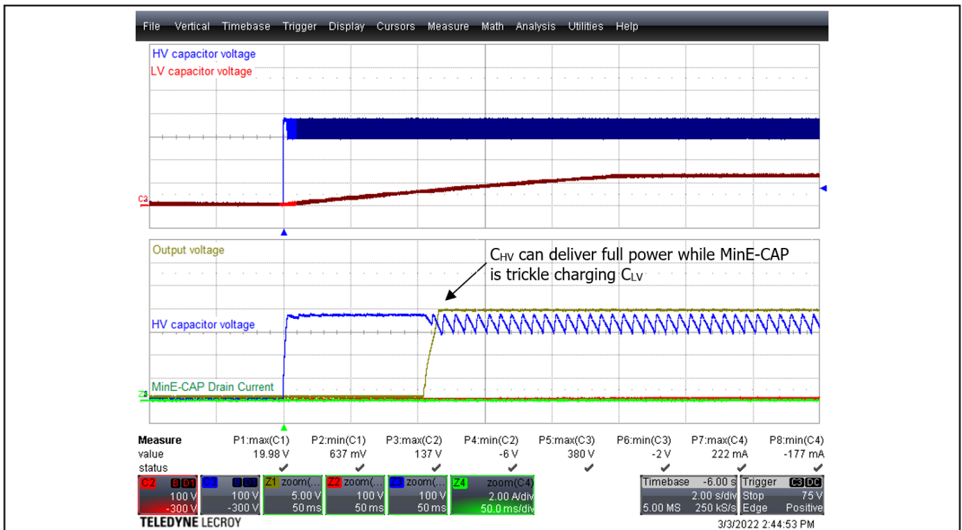
Figure 13. MinE-CAP IC Circuit Start-up Waveforms ( V_{IN} = 265 VAC, Load = 20 V, 3.25 A).
