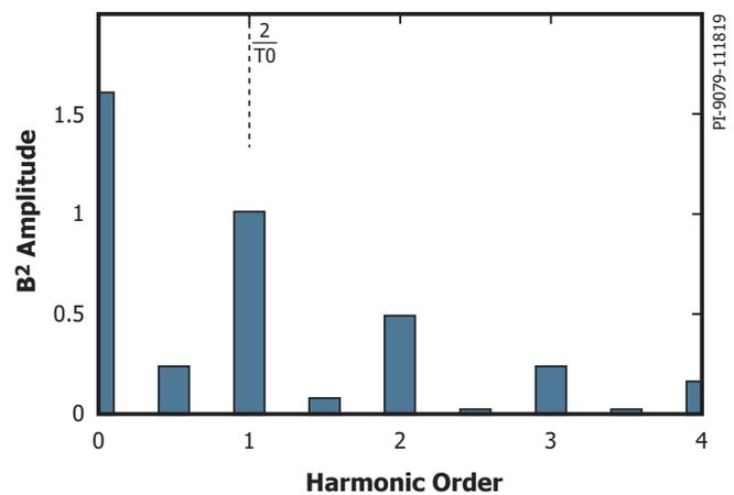
Figure 13. Two Output InnoMux Flyback Converter (VOR1  $\neq$  VOR2) –  $B^2(t)$  Harmonic Content.
