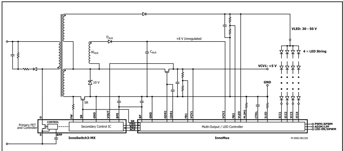
Figure 2. An Unregulated 8 V Auxiliary Supply ( $W_{AUX}$ ,  $D_{AUX}$  and  $C_{AUX}$ ) Reducing the Internal Dissipation in InnoMux.
