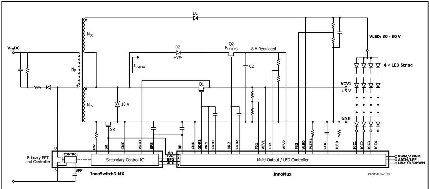
Figure 3. A Regulated 8 V Auxiliary Supply (D2, Q2) Supplying Power to InnoMux.
