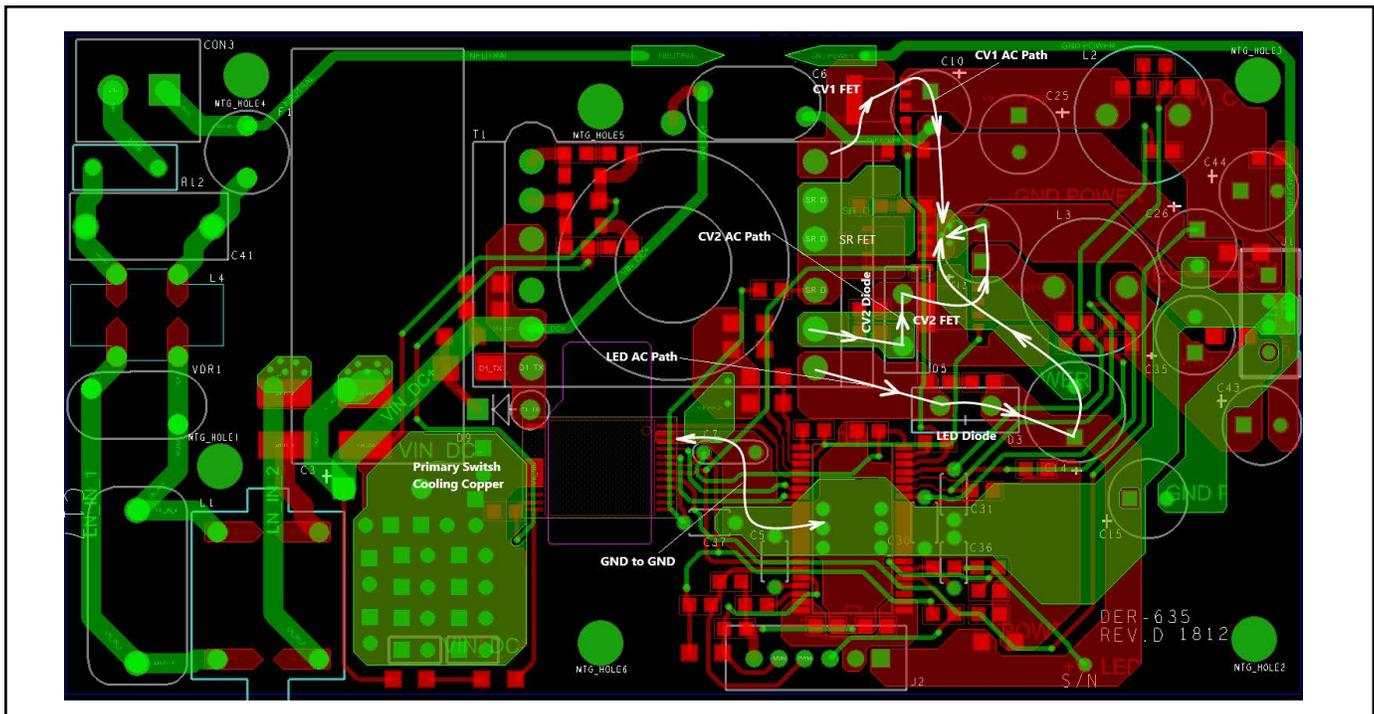
Figure 7. Two CV + 1 LED (CC) Output Converter – PCB Layout Example.
