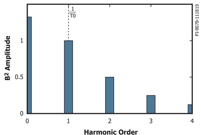
Figure 10. Discontinuous Flyback Converter  $B^2(t)$  Harmonic Content.
