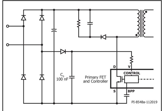
Figure 5. Fast Reset Circuit.
