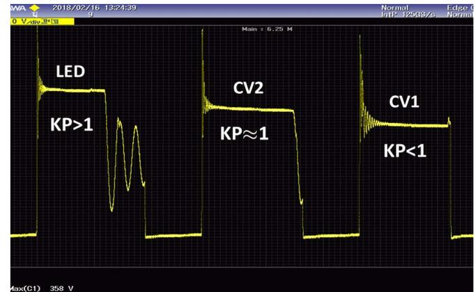
Figure 8. Primary Switch Drain Voltage of a Three-Output InnoMux Flyback Converter.
