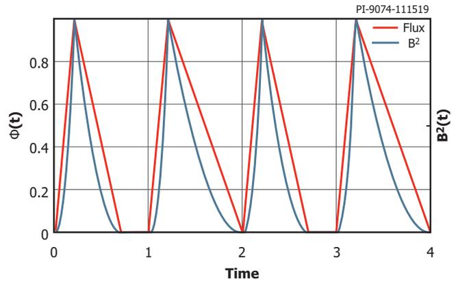
Figure 12. Normalized  $\Phi(t)$  and  $B^2(t)$  for a Two Output InnoMux Flyback Converter. (VOR1  $\neq$  VOR2)
