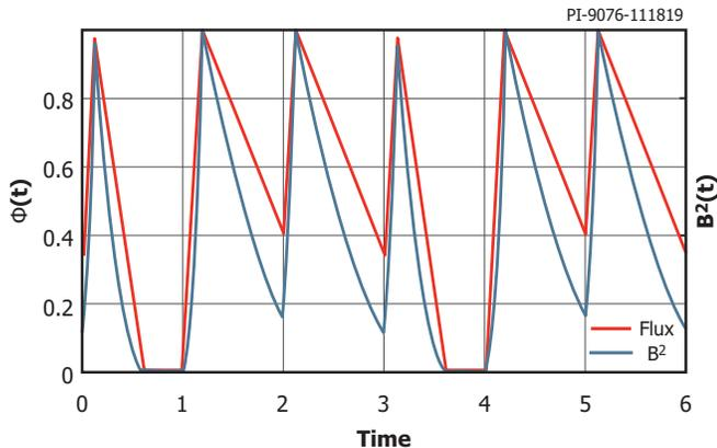
Figure 14. Normalized  $\Phi(t)$  and  $B^2(t)$  for a Two Output InnoMux Flyback Converter. (VOR1  $\neq$  VOR2; CC – DCM, CV – CCM)
