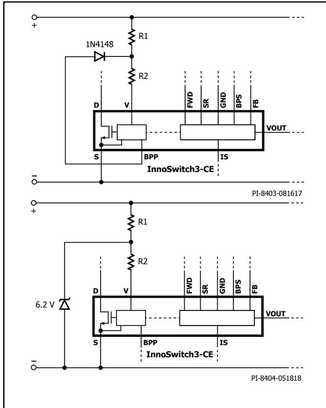
Figure 4. Above – Line OVP Only; Below – Line UVP Only.
