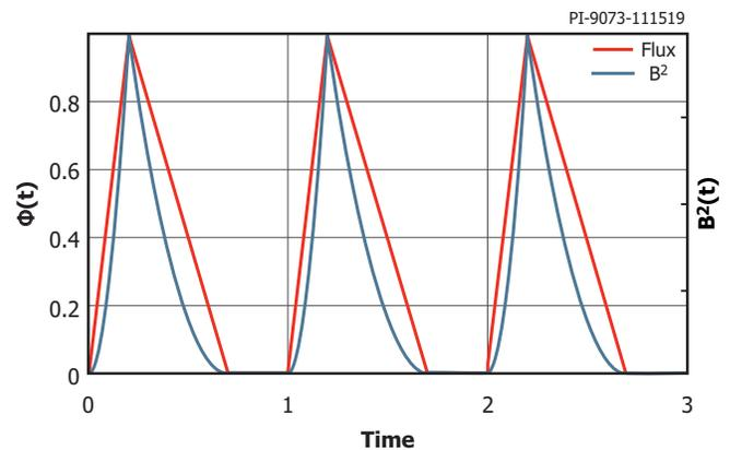
Figure 9. Normalized Magnetic Flux  $\phi(t)$  and Flux Density Squared  $B^2(t)$  for a Discontinuous Flyback Converter.
