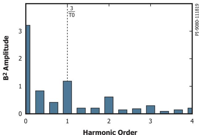
Figure 15. Two Output InnoMux Flyback Converter  $B^2(t)$  Harmonic Content (VOR1  $\neq$  VOR2; CC – DCM, CV – CCM).
