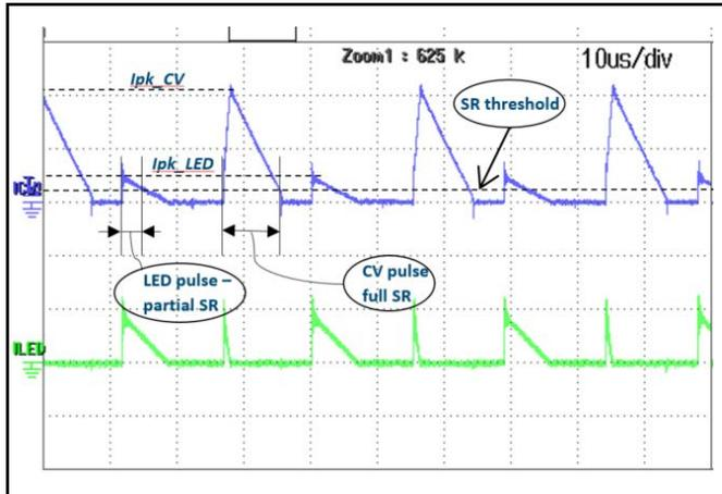
Figure 6. Typical SR and CC Winding Current Waveform.
