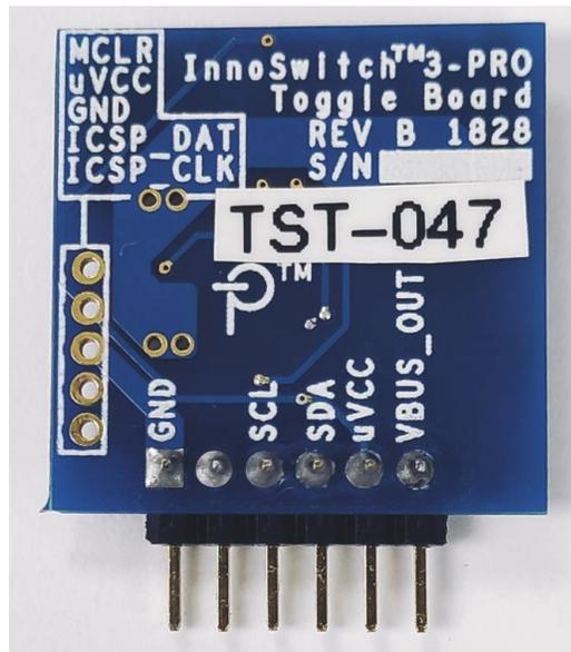
**Figure 2** – Bottom view of InnoSwitch3-Pro Toggle Board.
