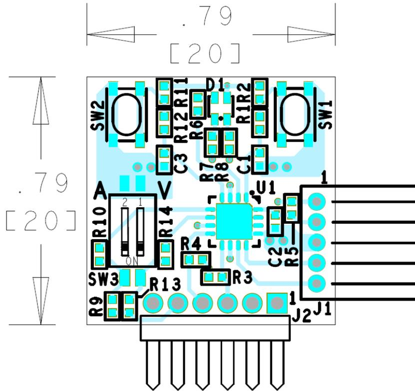
Figure 4 – PCB Top Layout.
