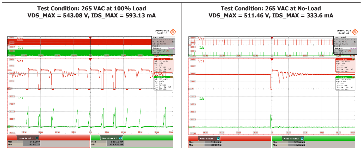
Figure 59. Primary Drain MOSFET Waveforms at 265 VAC Steady-state Operation 100% and No-Load Conditions.
