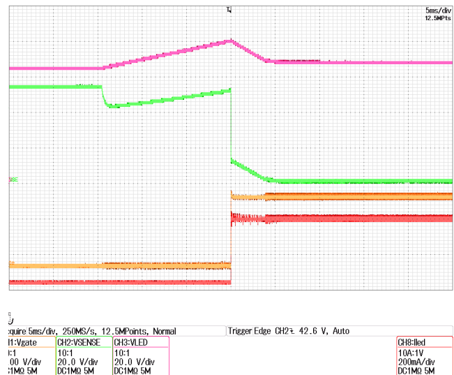
Figure 12. At LED Turn-On, LED Voltage Ramps up to Maximum Trimmed V_{LED} .
