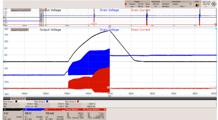
Figure 133 – 420 VAC 50 Hz Output Short. Full Load.
