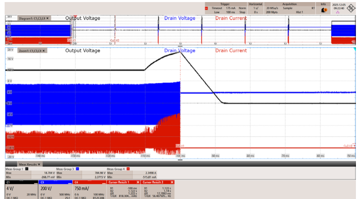
Figure 137 – 420 VAC 50 Hz. Full Load.
