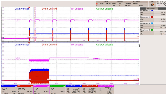
Figure 124 – 90 VAC 60 Hz. Output Short.
