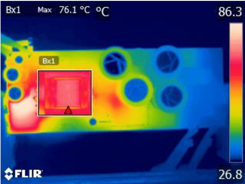
Figure 120 – 420 VAC 50 Hz. Top Side Discrete Component Thermals.
