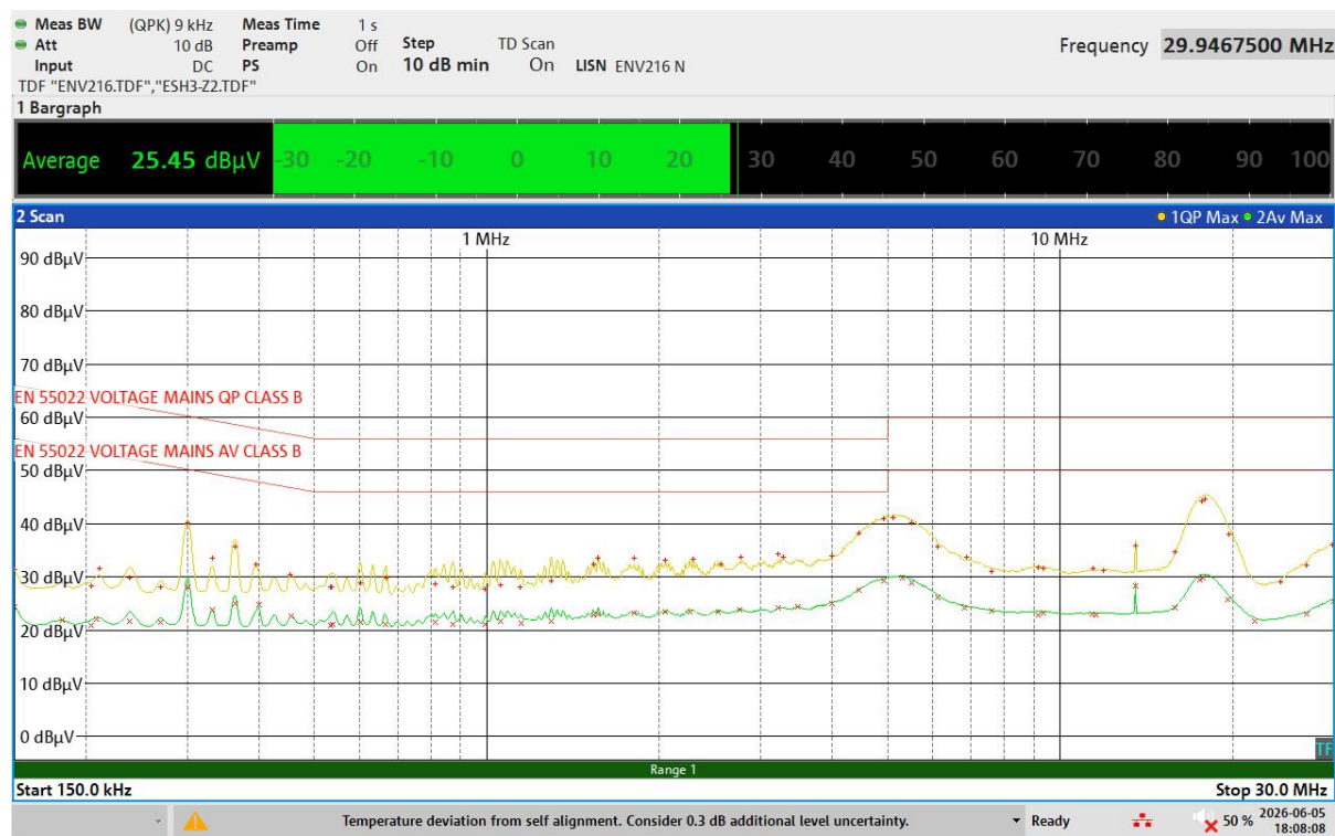
Figure 88 – Floating Ground EMI at 230 VAC b/w Input Lines A and B, Neutral
