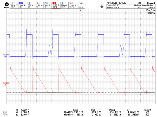
Figure 98 – Rectifier Diode Voltage and Current. 400 VDC, 1.3 A Load, -40 °C Ambient. CH2: V_{KA, D100} , 100 V / div. CH6: I_{D100} , 2.0 A / div. Time: 10 μs / div.
