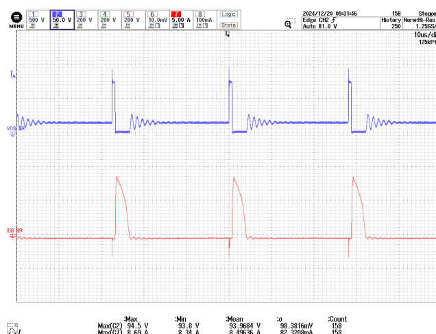
Figure 116 – SR FET Drain Voltage and Current. 800 V DC , Full Load. CH2: V DS,SR , 50 V / div. CH7: I D,SR , 5 A / div. Time: 10 μs / div.
