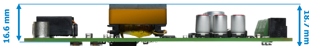
Figure 4 – Populated Circuit Board, Side.
