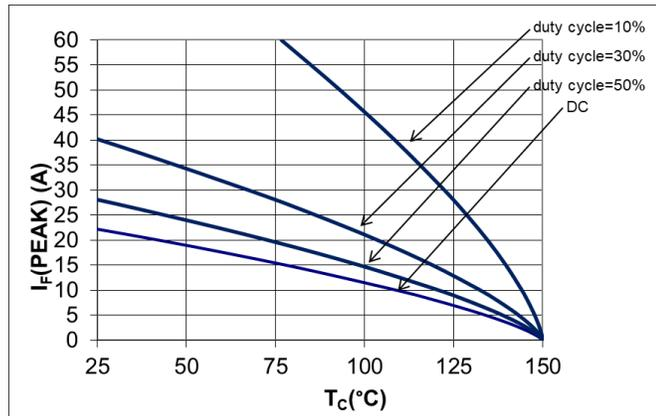
**Figure 9.  $I_F(\text{PEAK})$  vs  $T_C$ ,  $f = 70 \text{ kHz}$**
