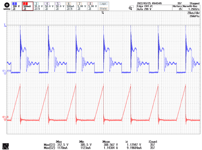
Figure 40 – INN3947CQ Drain Voltage and Current. 60 V DC , 1.333 A Load. CH1: V DS , 100 V / div. CH2: I D , 500 mA / div. Time: 10 μs / div.
