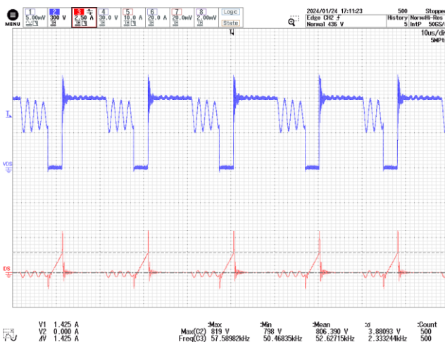
Figure 53 – INN3949CQ Drain Voltage and Current. 190 VDC, 5 A Load. CH2: V_{DS, INNO} , 300 V / div. CH3: I_{DS, INNO} , 2.5 A / div. Time: 10 \mu s / div.
