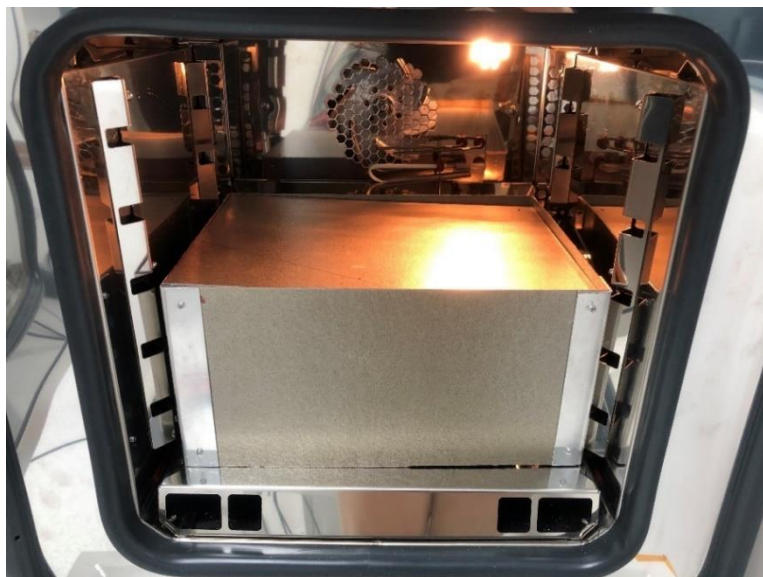
Figure 18 – Unit Under Test Placed Inside a Box to Eliminate the Effect of Airflow.
