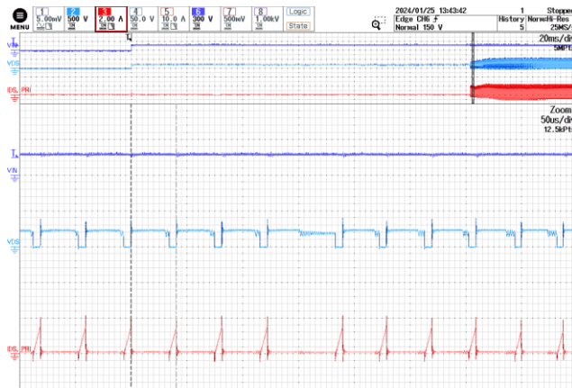
Figure 38 – INN3949CQ Drain Voltage and Current. 190 VDC, 2.8 \Omega Load. CH6: V_{IN} , 300 V / div. CH2: V_{OUT} , 500 V / div. CH3: I_{OUT} , 2 A / div. Time: 20 ms / div.
