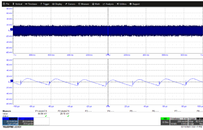
Figure 85 – 230 VAC Input, 50% Load V_{OUT} , 20 mV / div., 200 ms / div. Zoom: 20 \mu s Voltage Ripple: 44.8 mVpp
