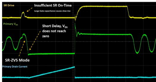
**Fig. 13 Insufficient SR on-time**
