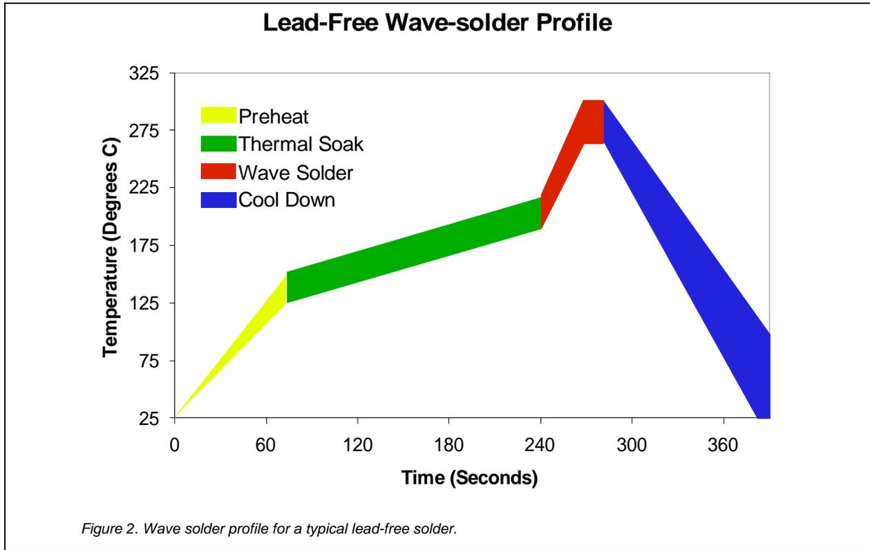
lead-free solder profile is noticeably longer than the equivalent stage for the leaded solder. The longer soak time is required to ensure that the components to be soldered have reached their higher pre-solder temperature.
