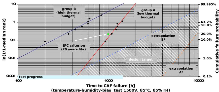
Figure 7 Weibull plot of CAF test data after 1450h
