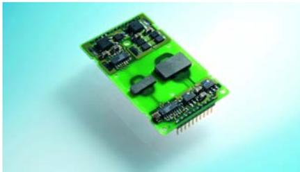
Figure 3 Planar transformer 1.7kV gate driver delivering 22W output power at 44 x 74 mm<sup>2</sup>, delay time 100ns, switching frequency DC to 250kHz (all data valid for unforced convection)
