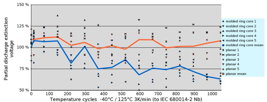
Figure 4 Accelerated ageing behavior of planar and wire-wound transformers
