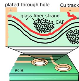
Figure 5 Formation of conductive filaments in FR4 material (schematic)
