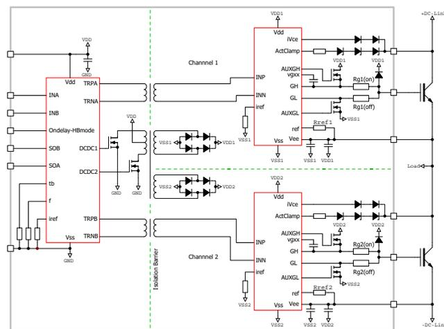
Figure 2 Schematic of the 2SD421 half bridge driver for PrimePACK modules
