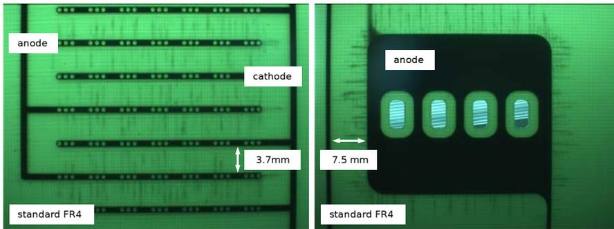
Figure 6 Standard FR4 PCB after 730h CAF testing at 1500V, 85°C and 85% rH
