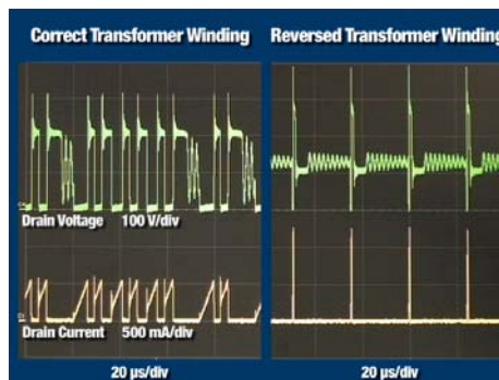
RD-91 drain current and voltage waveforms – with and without reversed winding
