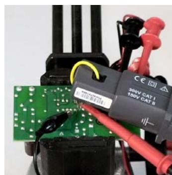
Connection of voltage and current probes
