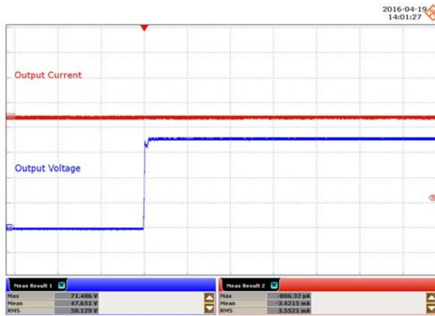
Figure 61 – 90 VAC, Open Load, Open Load Start-up. Upper: I_{OUT} , 50 mA / div. Lower: V_{OUT} , 20 V / div., 4 s / div.
