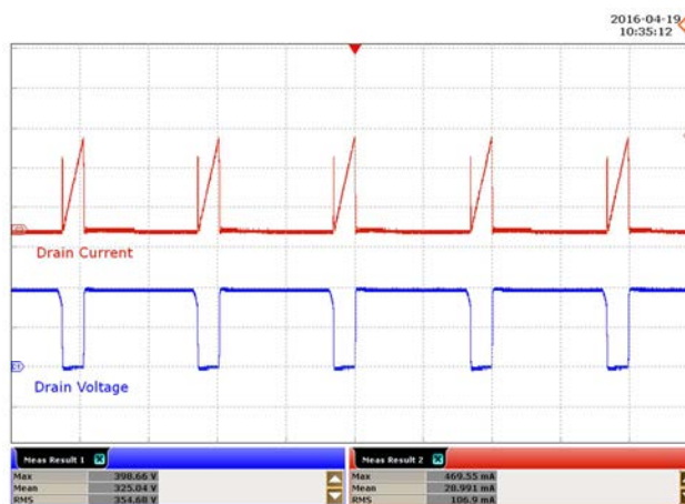
Figure 50 – 300 VAC, 60 V LED Load. Upper: I_{DRAIN} , 200 mA / div. Lower: V_{DRAIN} , 200 V / div., 5 us /div.
