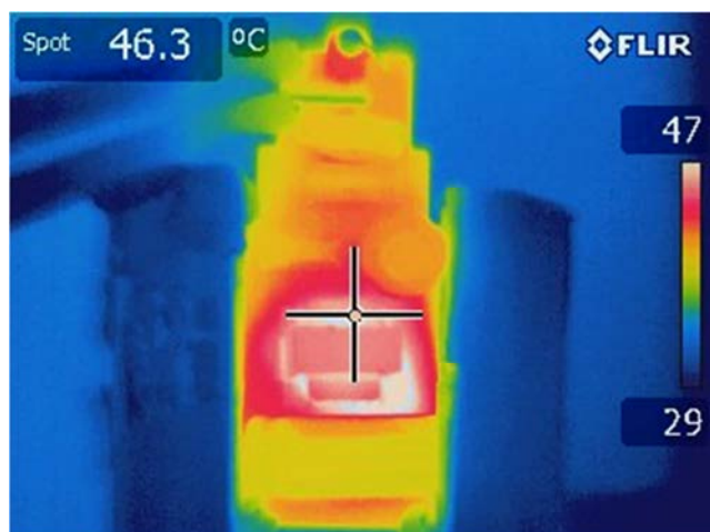
Figure 16 – 115 VAC, 60 V LED Load. Spot 1: Inductor (T1): 46.3 °C.
