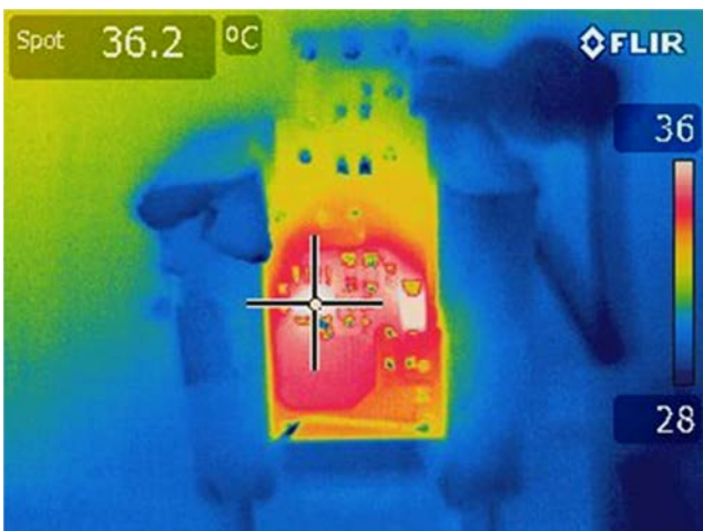
Figure 18 – 115 VAC, Output Shorted. Spot 1: LYT1603D (U1): 36.2 °C.
