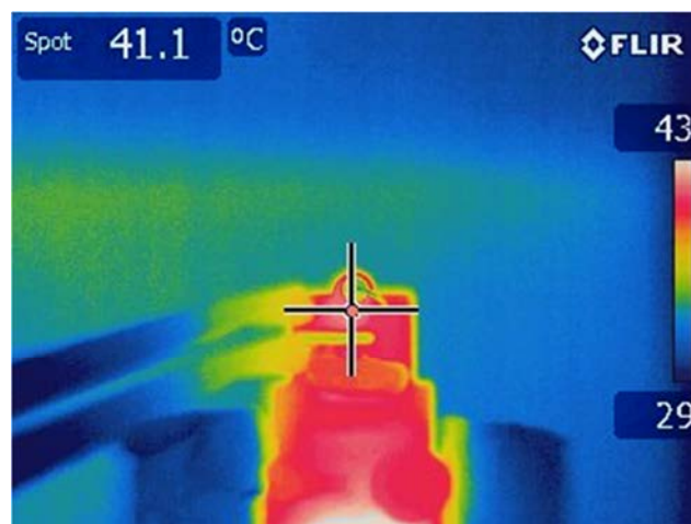
Figure 17 – 115 VAC, 60 V LED Load. Spot 1: Fusible Resistor (RF1): 41.1 °C.
