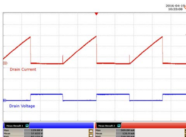
Figure 48 – 90 VAC, 60 V LED Load. Upper: I_{DRAIN} , 200 mA / div. Lower: V_{DRAIN} , 200 V / div., 5 us /div.
