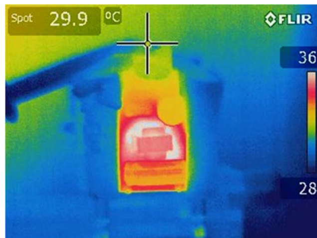
Figure 21 – 115 VAC, 60V Output Shorted. Spot 1: Fusible Resistor (RF1): 29.9 °C.
