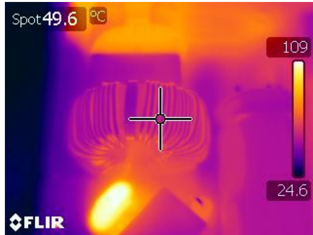
Figure 60 – Common Mode Choke (L1), 115 VAC Input, 100% Load, Room Temperature.
