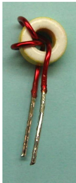
Figure 16 – Finished Part, Front View. Tin Leads to within ~ 1/8" of Toroid Body.
