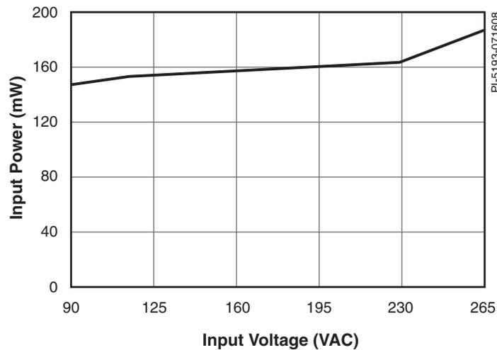
Figure 2. No-load Input Power vs. Line Voltage.
