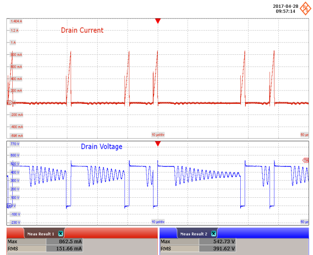
Figure 67 – 230 VAC 50 Hz, Full Load Normal Upper: I_{DRAIN} , 200 mA / div. Lower: V_{DRAIN} , 100 V / div., 10 \mu s / div.
