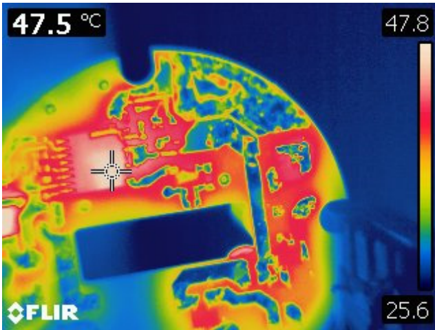
Figure 25 – 115 VAC 60 Hz, Full Load. InnoSwitch-CH (U1): 47.5 °C
