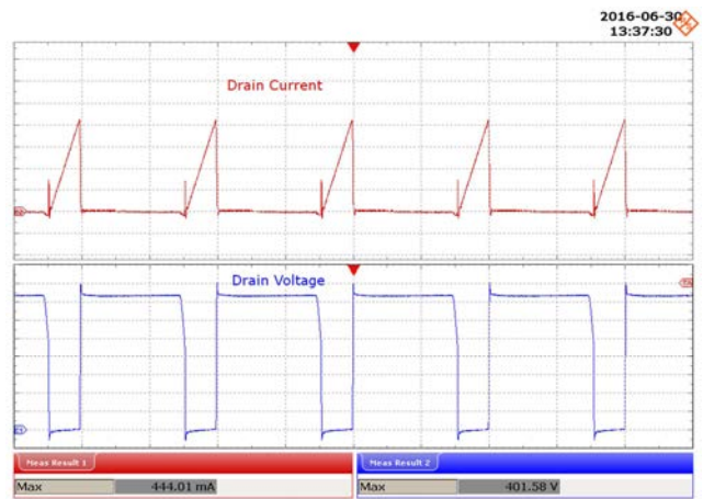
Figure 63 – 265 VAC, 84 V LED Load Upper: I_{DRAIN} , 100 mA / div. Lower: V_{DRAIN} , 50 V / div., 5 \mu s / div.
