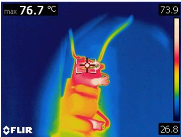
Figure 26 – 230 VAC, 84 V LED Load, Spot 1: Damper Resistor (R10): 76.7 °C.
