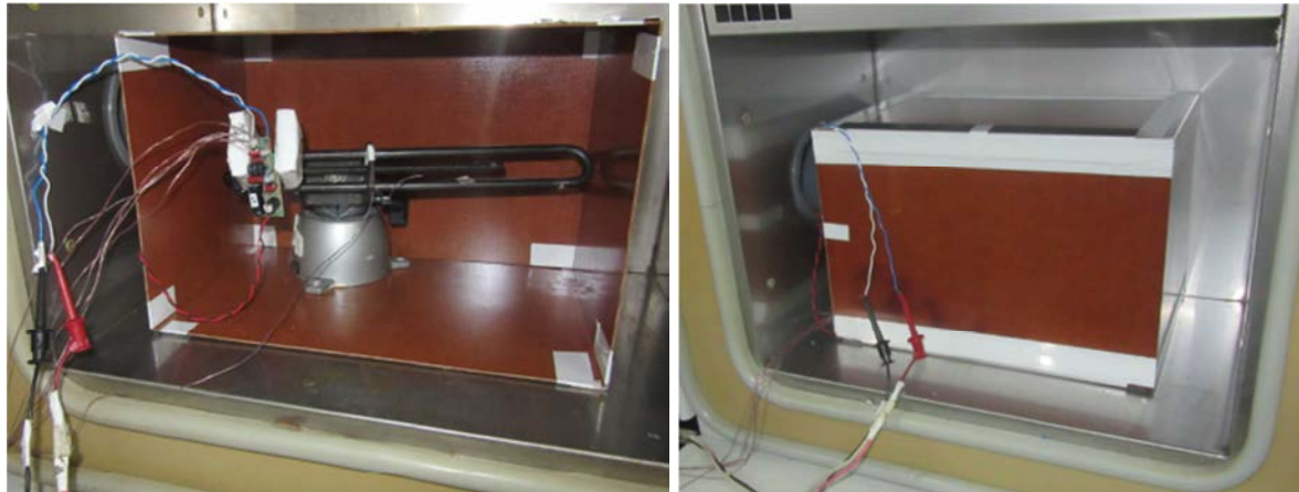
Figure 28 – Test Set-up Picture Thermal at 90 °C Ambient- Open Frame.
