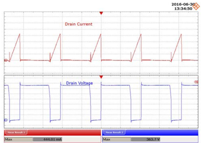
Figure 61 – 240 VAC, 84 V LED Load Upper: I_{DRAIN} , 100 mA / div. Lower: V_{DRAIN} , 50 V / div., 5 \mu s / div.
