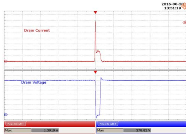
Figure 67 – 265 VAC, 84 V LED Load. Upper: I_{DRAIN} , 200 mA / div. Lower: V_{DRAIN} , 100 V / div., 1 \mu s / div.
