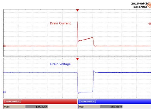
Figure 65 – 195 VAC, 84 V LED Load. Upper: I_{DRAIN} , 200 mA / div. Lower: V_{DRAIN} , 50 V / div., 1 \mu s / div.
