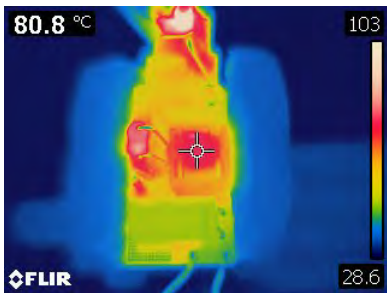
Figure 39 – Buck Inductor (T1) = 80.8 °C.
