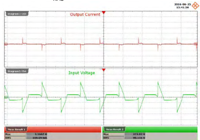
Figure 95 – 45° Conduction Angle. Upper: I_{IN} , 1 A / div. Lower: V_{IN} , 100 V / div., 10 ms / div. Peak V_{IN} : 272 V PK . V_{RMS} : 90 V.
