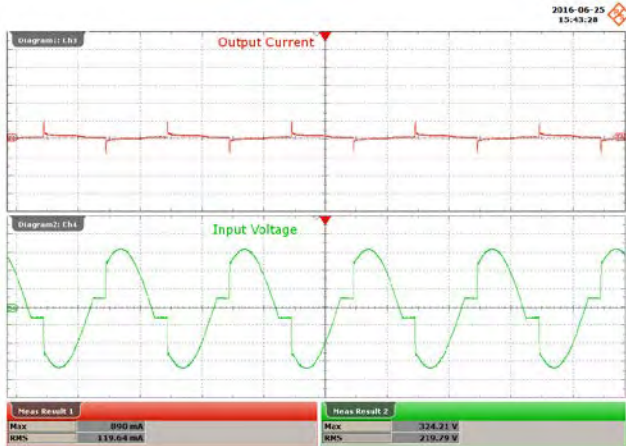
Figure 92 – 140° Conduction Angle. Upper: I_{IN} , 1 A / div. Lower: V_{IN} , 100 V / div., 10 ms / div. Peak V_{IN} : 324 V PK . V_{RMS} : 219 V.
