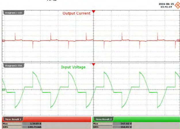
Figure 94 – 90° Conduction Angle. Upper: I_{IN} , 1 A / div. Lower: V_{IN} , 100 V / div., 10 ms / div. Peak V_{IN} : 348 V PK . V_{RMS} : 164 V.
