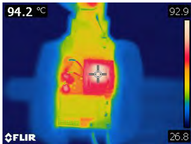
Figure 30 – Buck Inductor (T1) = 94.2 °C.
