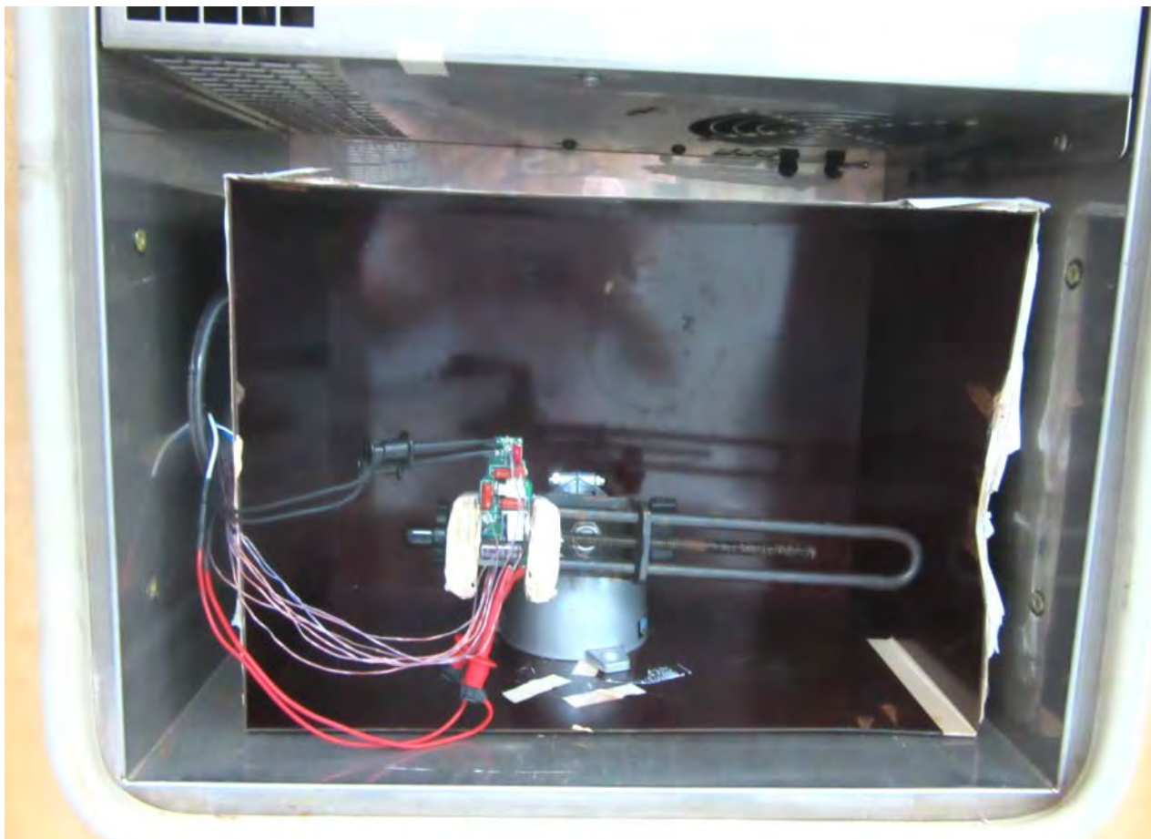
Figure 48 – Test Set-up Picture Thermal at 75 °C Ambient - Open Frame.
