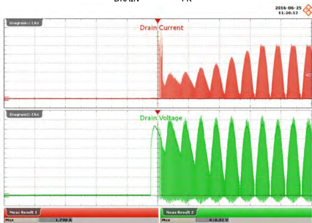
Figure 74 – 265 VAC, 52 V LED Load Upper: I_{DRAIN} , 200 mA / div. Lower: V_{DRAIN} , 100 V / div., 20 ms /div. Peak I_{DRAIN} : 1.8 A PK . Peak V_{DRAIN} : 418 V PK .
