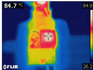
Figure 21 – Buck Inductor (T1) = 84.7 °C.
