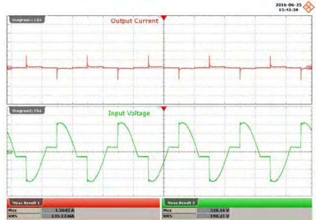
Figure 93 – 110° Conduction Angle. Upper: I_{IN} , 1 A / div. Lower: V_{IN} , 100 V / div., 10 ms / div. Peak V_{IN} : 328 V PK . V_{RMS} : 198 V.
