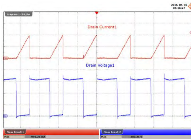
Figure 51 – 115 VAC, 60 V LED Load. Upper: I_{DRAIN} , 500 mA / div. Lower: V_{DRAIN} , 50 V / div., 10 \mu s / div.
