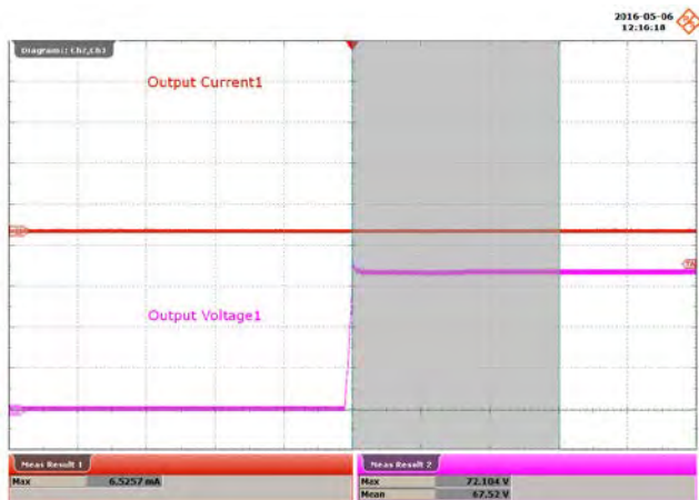
Figure 88 – 100 VAC, 60 V LED Load. Open Load_1 Start-up. Running Load_2 Start-up. Upper: I_{OUT} , 100 mA / div. Lower: V_{OUT} , 20 V / div., 4 s / div.
