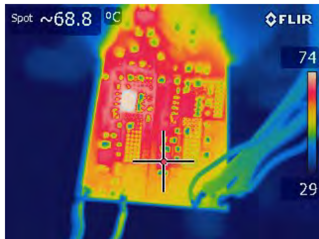
Figure 26 – 115 VAC, Output_2 Short. Spot 1: Flywheel Diode (D2): 68.8 °C.
