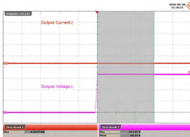
Figure 89 – 100 VAC, 60 V LED Load. Open Load_2 Start-up. Running Load_1 Start-up. Upper: I_{OUT} , 100 mA / div. Lower: V_{OUT} , 20 V / div., 4 s / div.
