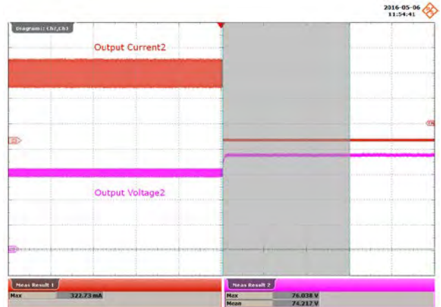
Figure 87 – 120 VAC, 60 V LED Load. Output 2 Running Open Load. Output 1 Normal Running. Upper: I_{OUT} , 100 mA / div. Lower: V_{OUT} , 20 V / div., 4 s / div.
