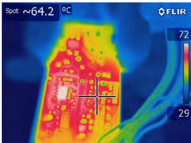
Figure 25 – 115 VAC, Output_2 Short. Spot 1: LYT1604D (U2): 64.2 °C.
