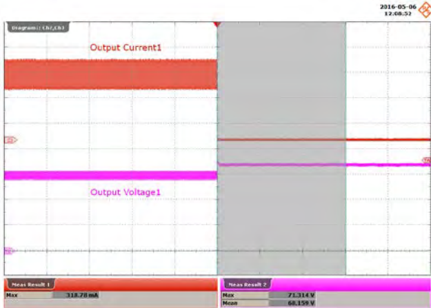
Figure 84 – 100 VAC, 60 V LED Load. Output 1 Running Open Load. Output 2 Normal Running. Upper: I_{OUT} , 100 mA / div. Lower: V_{OUT} , 20 V / div., 4 s / div.
