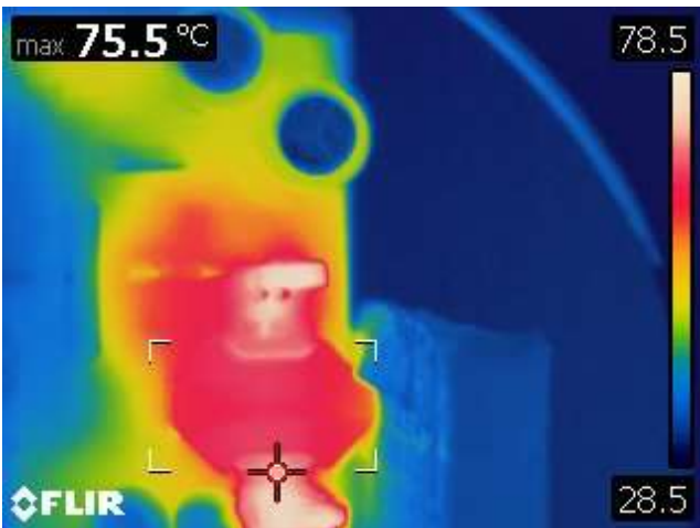
Figure 42 – Ambient = 27 °C. Secondary Diode = 75.5 °C.
