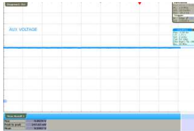
Figure 50 – 265 VAC, Full Load. V_{AUX} , 2 V / div., 10 ms / div. Measured Peak to Peak Voltage = 247 mV PK-PK . Measured Mean Voltage = 9.69 V.
