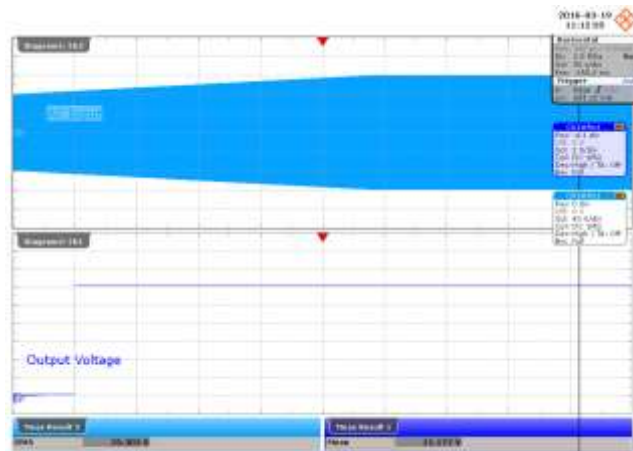
Figure 72 – 85 VAC, 60 Hz. Brown-in. Upper: V_{AC} , 40 V / div., 50 s / div. Lower: V_{OUT} , 2 V / div., 50 s / div.
