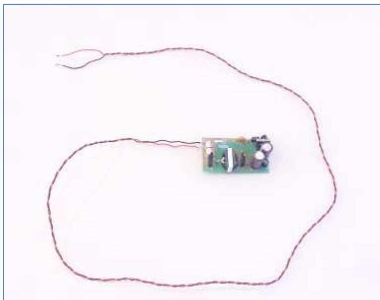
Figure 8 – Unit Under Test with the Equivalent 100 m \Omega Cable.
