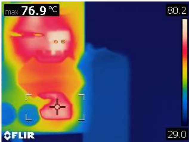
Figure 35 – Ambient = 27 °C. Secondary Diode = 76.9 °C.
