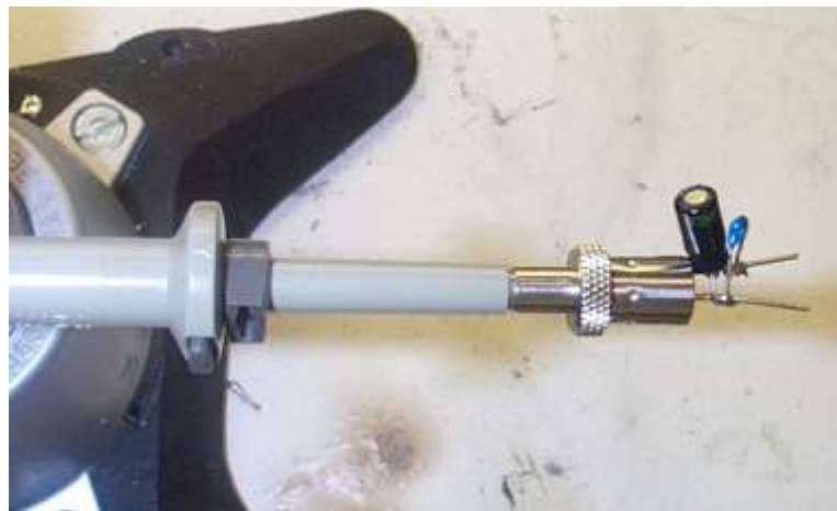
Figure 82 – Oscilloscope Probe with Probe Master ( www.probemaster.com ) 4987A BNC Adapter. (Modified with wires for ripple measurement, and two parallel decoupling capacitors added.)
