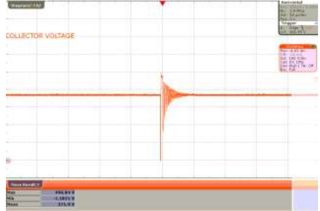
Figure 52 – 265 VAC, No-Load. V_{COL} , 100 V / div., 50 \mu s / div. Maximum Peak Collector Voltage = 496 V_{PK} .
