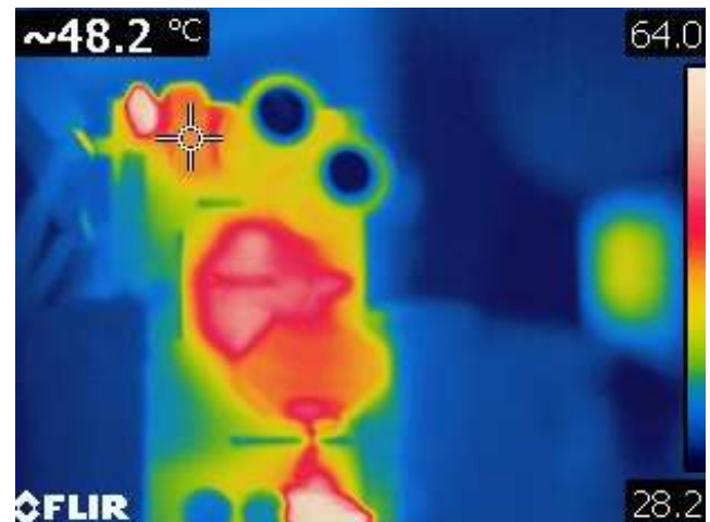
Figure 32 – Ambient = 27 °C. CMC Choke = 48.2 °C.
