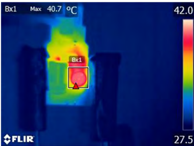
Figure 20 – 115 VAC, Output Short. Spot 1: Drum Choke (L2): 40.7 °C.
