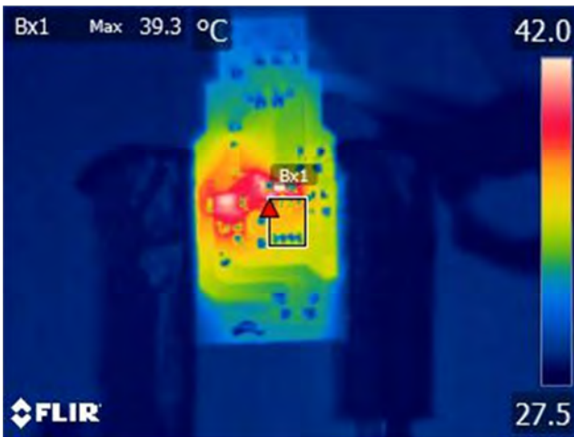
Figure 18 – 115 VAC, Output Short. Spot 1: LYT1603D (U1): 39.3 °C.
