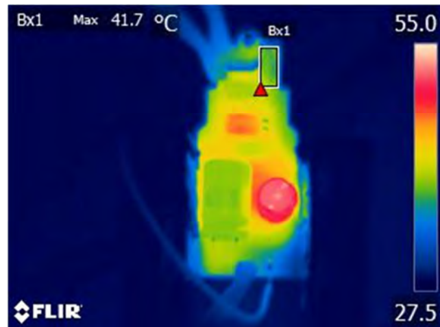
Figure 17 – 115 VAC, 52 V LED Load. Spot 1: Varistor (RV1): 41.7 °C.
