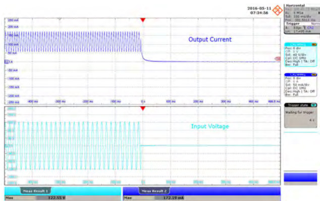
Figure 41 – 90 VAC, 52 V LED, Output Fall. Upper: I_{OUT} , 50 mA / div. Lower: V_{IN} , 40 V / div., 100 ms / div.
