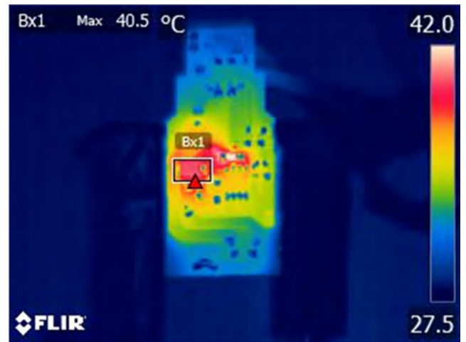
Figure 19 – 115 VAC, Output Short. Spot 1: Flywheel Diode (D1): 40.5 °C.
