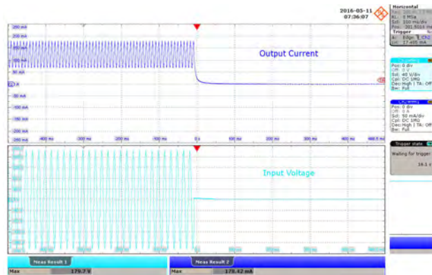
Figure 44 – 132 VAC, 52 V LED, Output Fall. Upper: I_{OUT} , 50 mA / div. Lower: V_{IN} , 40 V / div., 100 ms / div.
