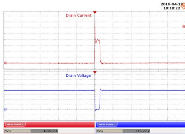
Figure 55 – 300 VAC, 120 V LED Load. Upper: I_{DRAIN} , 200 mA / div. Lower: V_{DRAIN} , 100 V / div., 1 \mu s /div.
