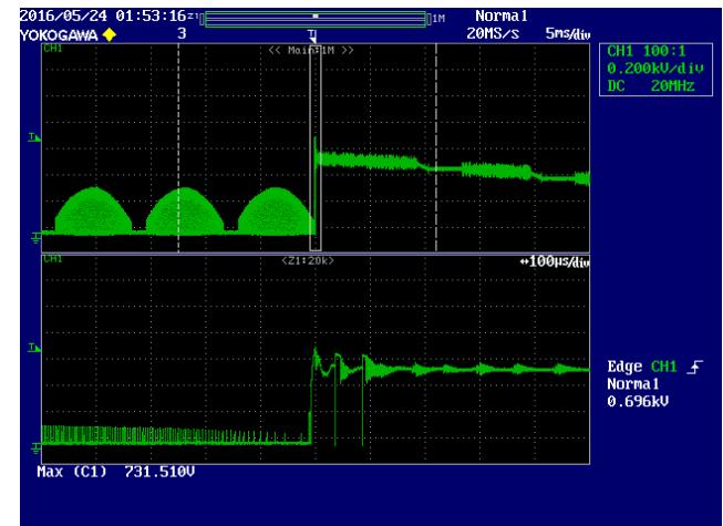
**Figure 78 – +1 kV Differential Surge, 0° Phase Angle.**
