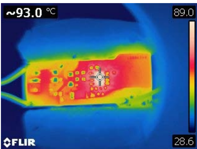
Figure 15 – 115 VAC, 67 V LED Load. Spot 1: LYT1604D (U1): 93 °C.
