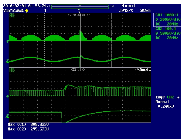
Figure 97 — (-)1 kV Ring Wave Surge, 90° Phase Angle. CH1: V_{DRAIN} , 100 V / div., 5 ms / div. Peak V_{DRAIN} : 308.33 V.
