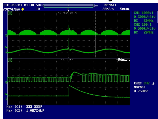
Figure 96 — (+)1 kV Differential Surge, 90° Phase Angle. CH1: V_{DRAIN} , 100 V / div., 5 ms / div. Peak V_{DRAIN} : 333.33 V.
