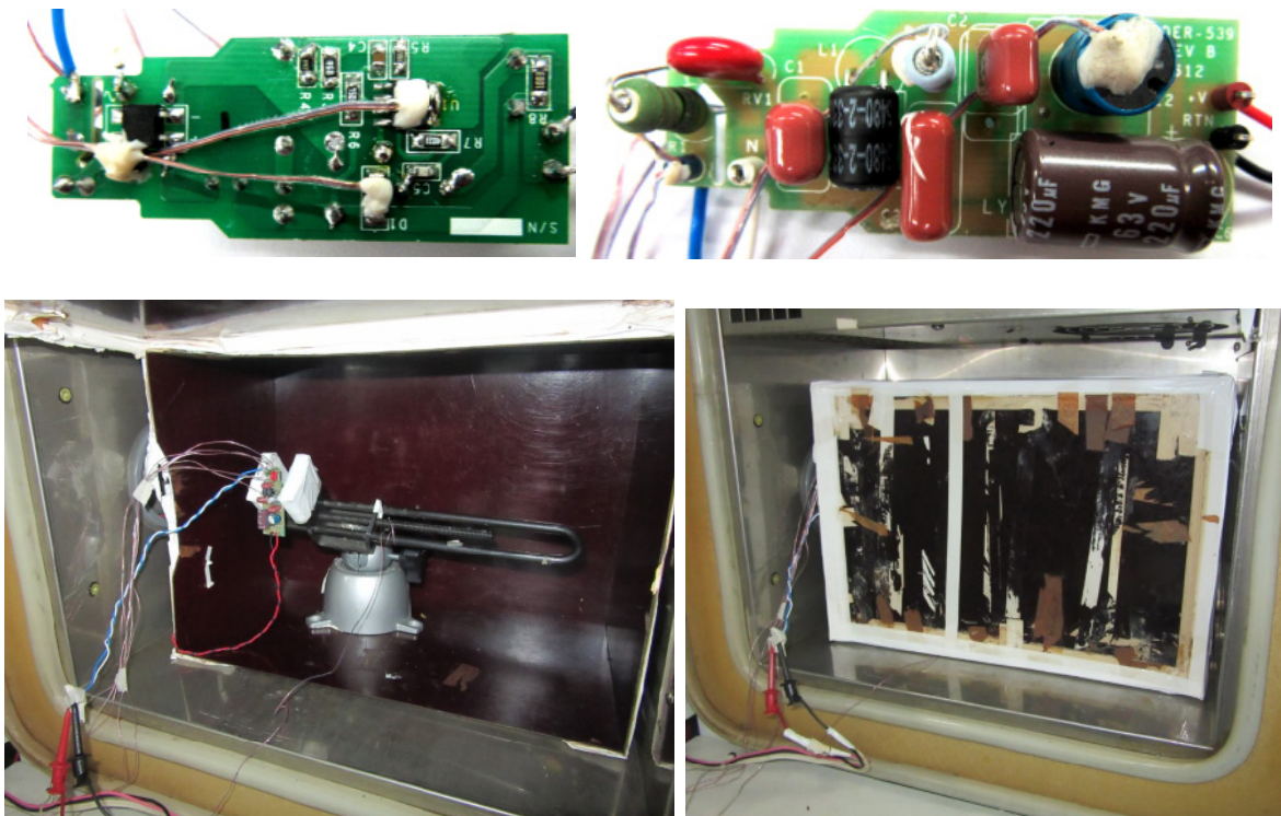
Figure 28 – Test Set-up Picture Thermal at 75 °C Ambient - Open Frame.
