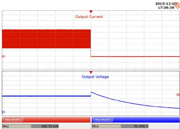
Figure 66 – 195 VAC, 72 V LED Load, Running Open Load. Upper: I_{OUT} , 40 mA / div. Lower: V_{OUT} , 20 V / div., 4 s / div.
