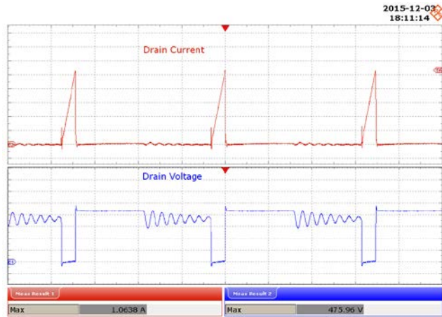
Figure 53 – 265 VAC, 72 V LED Load Upper: I_{DRAIN} , 200 mA / div. Lower: V_{DRAIN} , 100 V / div., 4 \mu s / div.
