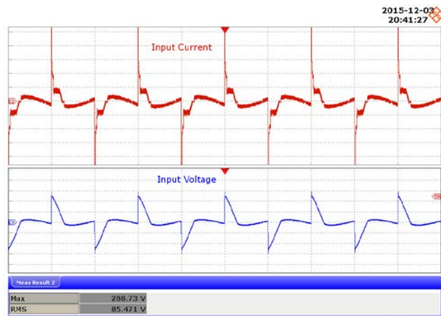
Figure 77 – 50° Conduction Angle. Upper: I_{IN} , 40 mA / div. Lower: V_{IN} , 100 V / div., 10 ms / div.
