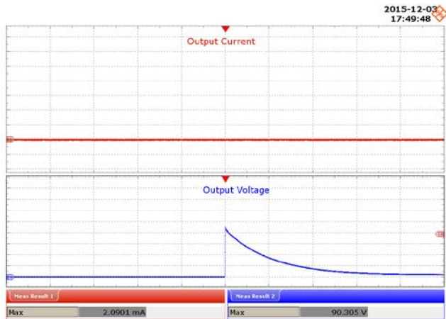
Figure 68 – 195 VAC, 72 V LED Load, Running Open Load. Upper: I_{OUT} , 40 mA / div. Lower: V_{OUT} , 20 V / div., 10 s / div.
