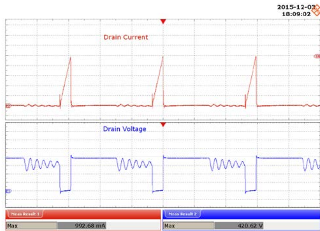
Figure 51 – 230 VAC, 72 V LED Load Upper: I_{DRAIN} , 200 mA / div. Lower: V_{DRAIN} , 100 V / div., 4 \mu s / div.
