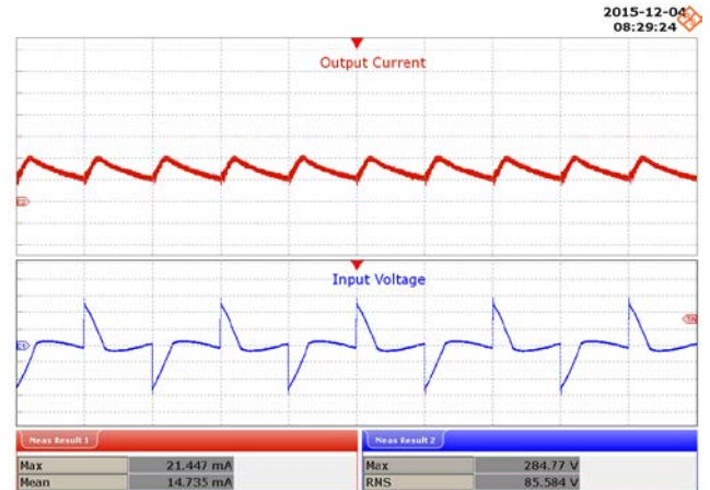
Figure 81 – 50° Conduction Angle. Upper: I_{OUT} , 10 mA / div. Lower: V_{IN} , 100 V / div., 10 ms / div.
