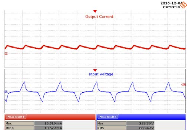
Figure 89 – 50° Conduction Angle. Upper: I_{OUT} , 10 mA / div. Lower: V_{IN} , 100 V / div., 10 ms / div.
