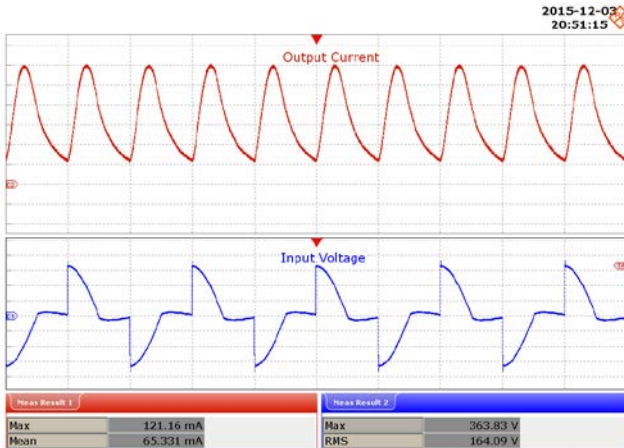
Figure 80 – 90° Conduction Angle. Upper: I_{OUT} , 20 mA / div. Lower: V_{IN} , 100 V / div., 10 ms / div.
