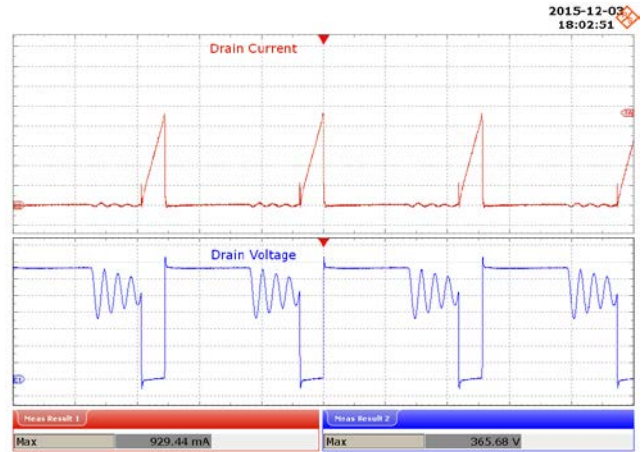
Figure 47 – 195 VAC, 72 V LED Load. Upper: I_{DRAIN} , 200 mA / div. Lower: V_{DRAIN} , 50 V / div., 4 μs / div.
