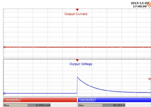
Figure 69 – 265 VAC, 72 V LED Load, Running Open Load. Upper: I_{OUT} , 40 mA / div. Lower: V_{OUT} , 20 V / div., 10 s / div.
