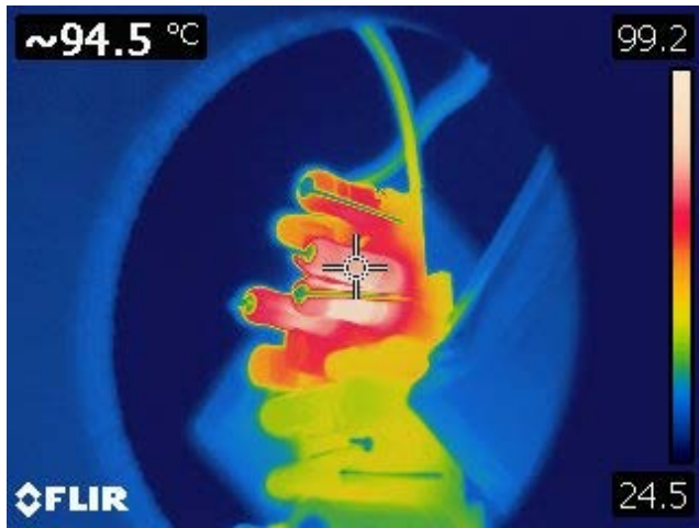
Figure 26 – 230 VAC, 72 V LED Load. Spot 1: Bleeder (R32): 94.5 °C.
