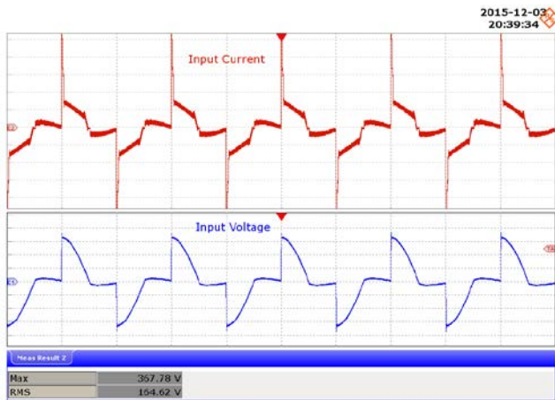
Figure 76 – 90° Conduction Angle. Upper: I_{IN} , 40 mA / div. Lower: V_{IN} , 100 V / div., 10 ms / div.
