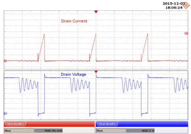
Figure 49 – 220 VAC, 72 V LED Load. Upper: I_{DRAIN} , 200 mA / div. Lower: V_{DRAIN} , 50 V / div., 4 μs / div.
