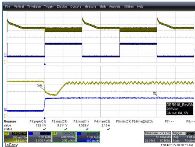
Figure 17 – Transient Response 265 VAC, 0-2 A Load Step. Min. V OUT : 4.529 V, Max. V OUT : 5.311 V. CH1(Olive): V OUT , 0.2 V / div. CH3(Blue): I OUT , 1 A / div. 50 ms / div., 200 \mu\text{s} / div. (Zoom).
