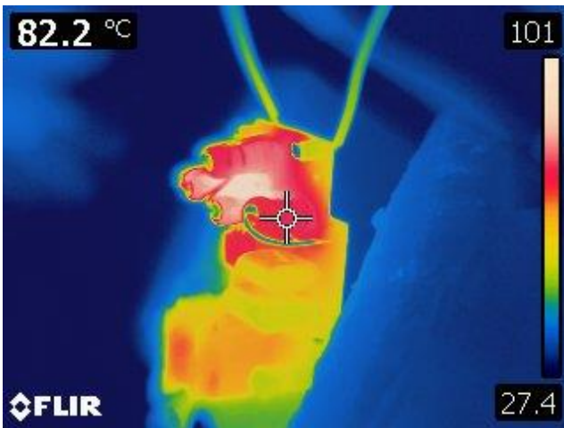
Figure 24 – 120 VAC, 72 V LED LOAD. Spot 1: Damper Resistor (R7): 82.2 °C.
