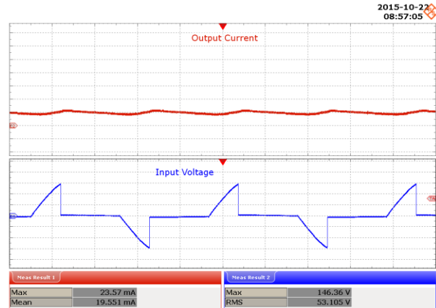
Figure 81 – 60° Conduction Angle. Upper: I_{OUT} , 20 mA / div. Lower: V_{IN} , 50 V / div., 5 ms / div.
