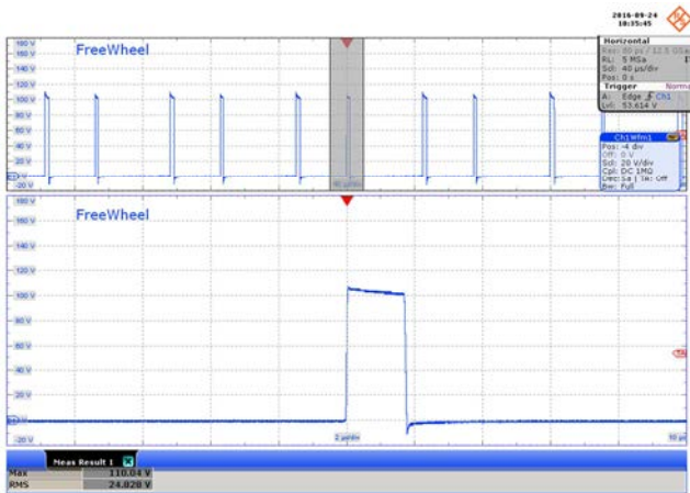
Figure 30 – 85 VAC Input. V_{FWL} , 20 V / div, 40 \mu s / div. Zoom: 2 \mu s / div. I_{FWLMAX} : 110.04 V.
