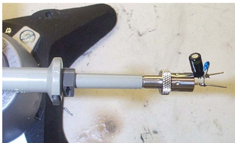
Figure 12 – Oscilloscope Probe with Probe Master ( www.probemaster.com ) 4987A BNC Adapter. (Modified with wires for ripple measurement, and two parallel decoupling capacitors added)
